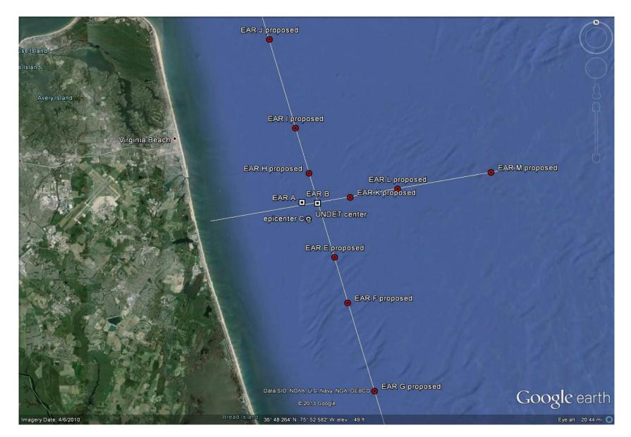
Figure 43. Spatial configuration of three linear coastal EAR arrays (north, east and south) that will be used during the second year of the project. Only one 4-EAR linear array will be deployed at any given time.
