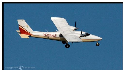
Figure 1. Partenavia twin-engine aircraft flown for aerial surveys. Line-transects were flown at 1000 ft altitude; focal observations were flown in circles from 1200-1500 ft. altitude and 0.5-1 km radial distance (outside the sound cone of plane) to avoid disturbance of marine mammals
