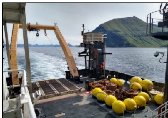
Figure 2. Back deck of NOAA Ship Oscar Dyson during EcoFOCI fall mooring cruise, showing the A-frame and blocks used in mooring deployment and recovery.
