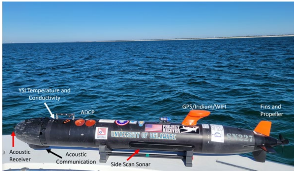
Figure 4. REMUS 100 Autonomous Underwater Vehicle equipped with side scan sonar, acoustic telemetry receiver and environmental sensors utilized to detect Gulf Sturgeon.
