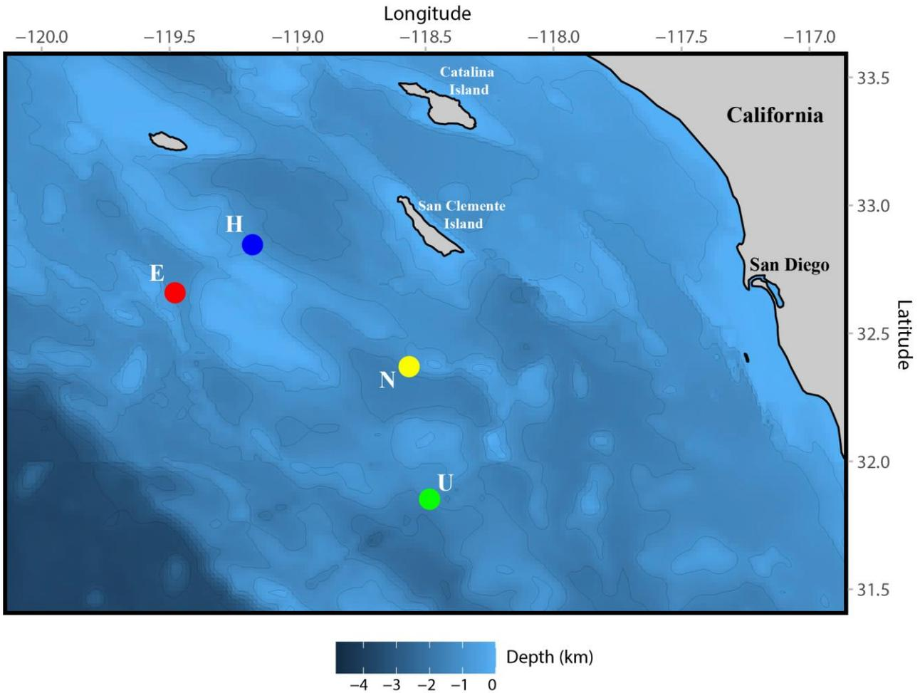
**Figure 1. Locations of High-frequency Acoustic Recording Package (HARP) deployment sites E, H, N, and U (circles) in the SOCAL study area from November 2018 through May 2020. Color indicates bathymetric depth. Contour lines represent 500 m depth increments.**
