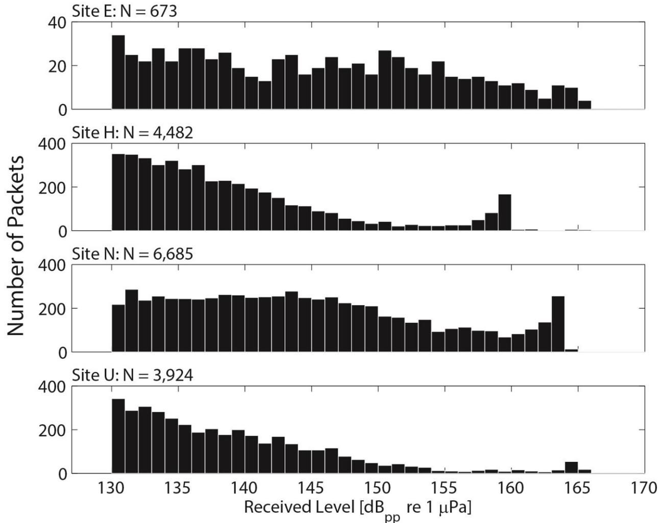
**Figure 22. MFA sonar packet peak-to-peak received level distributions for sites E, H, N, and U. The total number of packets detected at each site is given in the upper left corner of each panel. Instrument clipping levels are reached around 165 dB<sub>pp</sub> re 1  $\mu$ Pa, except for deployment 67 at site H where clipping levels were around 160 dB<sub>pp</sub> re 1  $\mu$ Pa. Note the vertical axes are at different scales with site E being smaller.**
