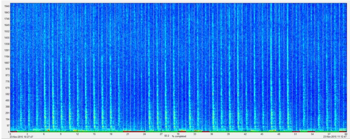
**Figure 9. Explosions previously detected at site H in the analyst verification stage where events are concatenated into a single spectrogram. Green along the bottom indicates true and red indicates false detections.**
