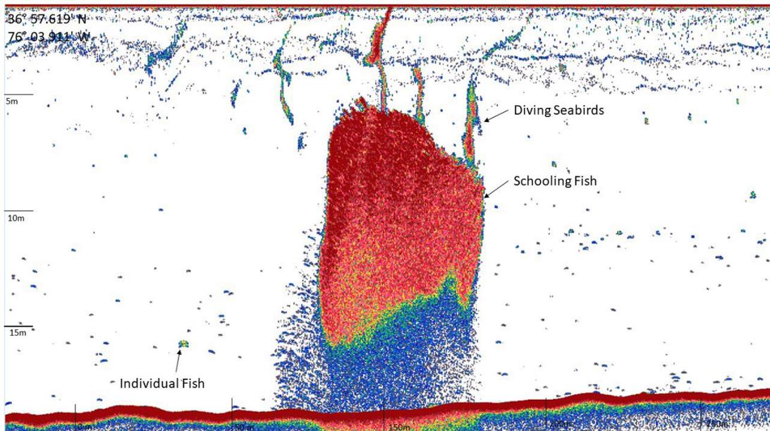
Figure 8. Example echogram showing a large fish school in the water column.
