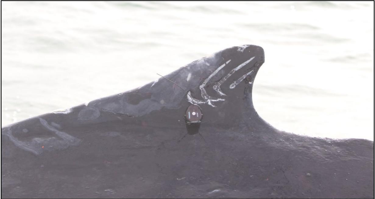
Figure 4. LIMPET SPLASH10-F tag on a humpback whale immediately after deployment.
