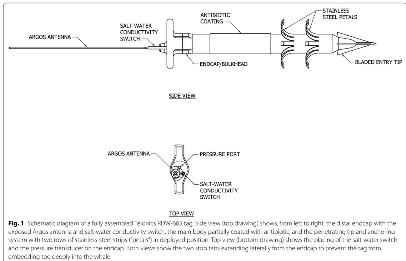
consists of two rows of ten outwardly curved metal strips (each strip was 3.2 cm long  $\times$  0.6 cm wide) mounted on the main body at the nose cone (proximal) end (Fig. 1). Total tag weight is approximately 300 g.
