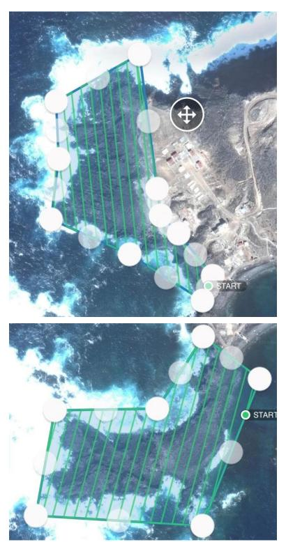
**Figure 3.** Drone flight plans for the main peninsula (bottom panel) and west side (top panel) of Punta Sur (southernmost point) at Guadalupe Island. Parallel green lines indicate the drone flight path, and white circles represent nodes for creating the transect area (blue/green outline).
