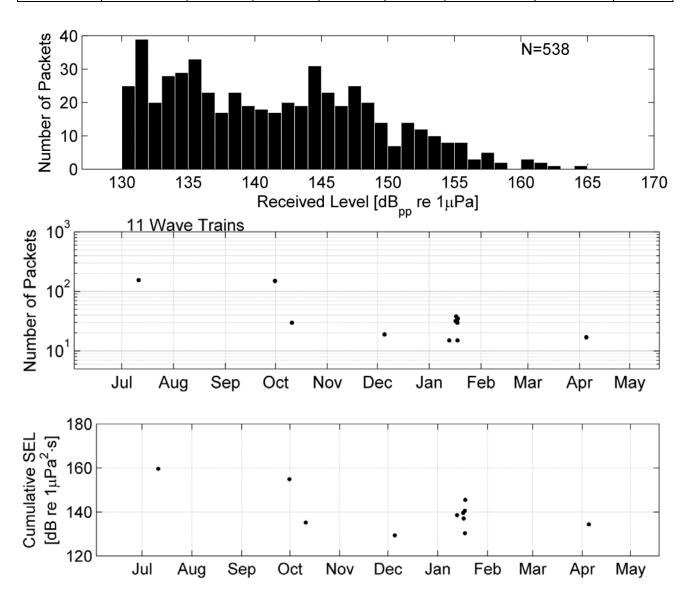
Figure 27. Top: Distribution of received levels (RL) of detected MFA packets. Center: Number of MFA packets detected in each wave train exceeding the minimum RL threshold (130 dBpp re  $1\mu$  Pa). Bottom: Cumulative sound exposure levels (CSEL) associated with each wave train.
