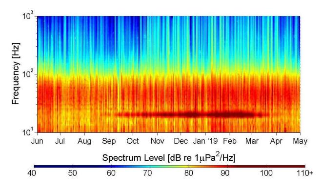
Figure 14. Long-term spectrograms using daily-averaged spectra for NFC Site A from June 2018 to May 2019.
