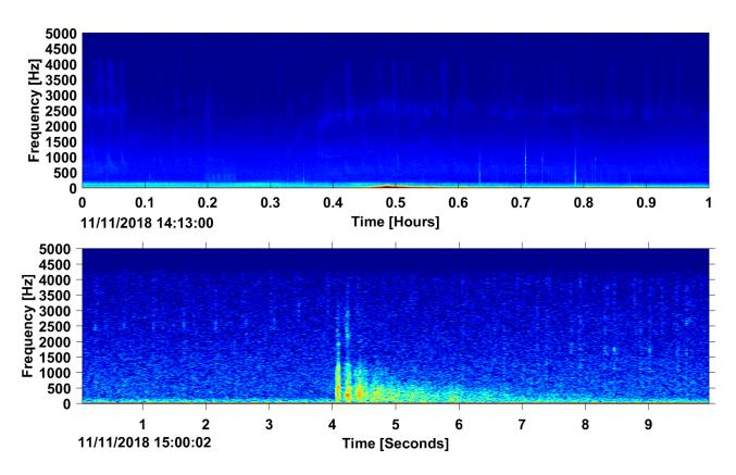
Figure 12. Explosions in LTSA (top) and spectrogram (bottom) recorded at NFC Site A, November 2018.
