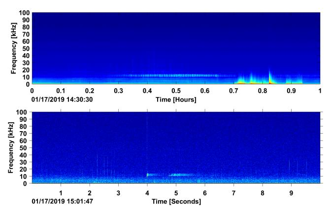
Figure 11. High-Frequency Active (HFA) sonar in LTSA (top) and spectrogram (bottom) recorded at NFC Site A, January 2019.
