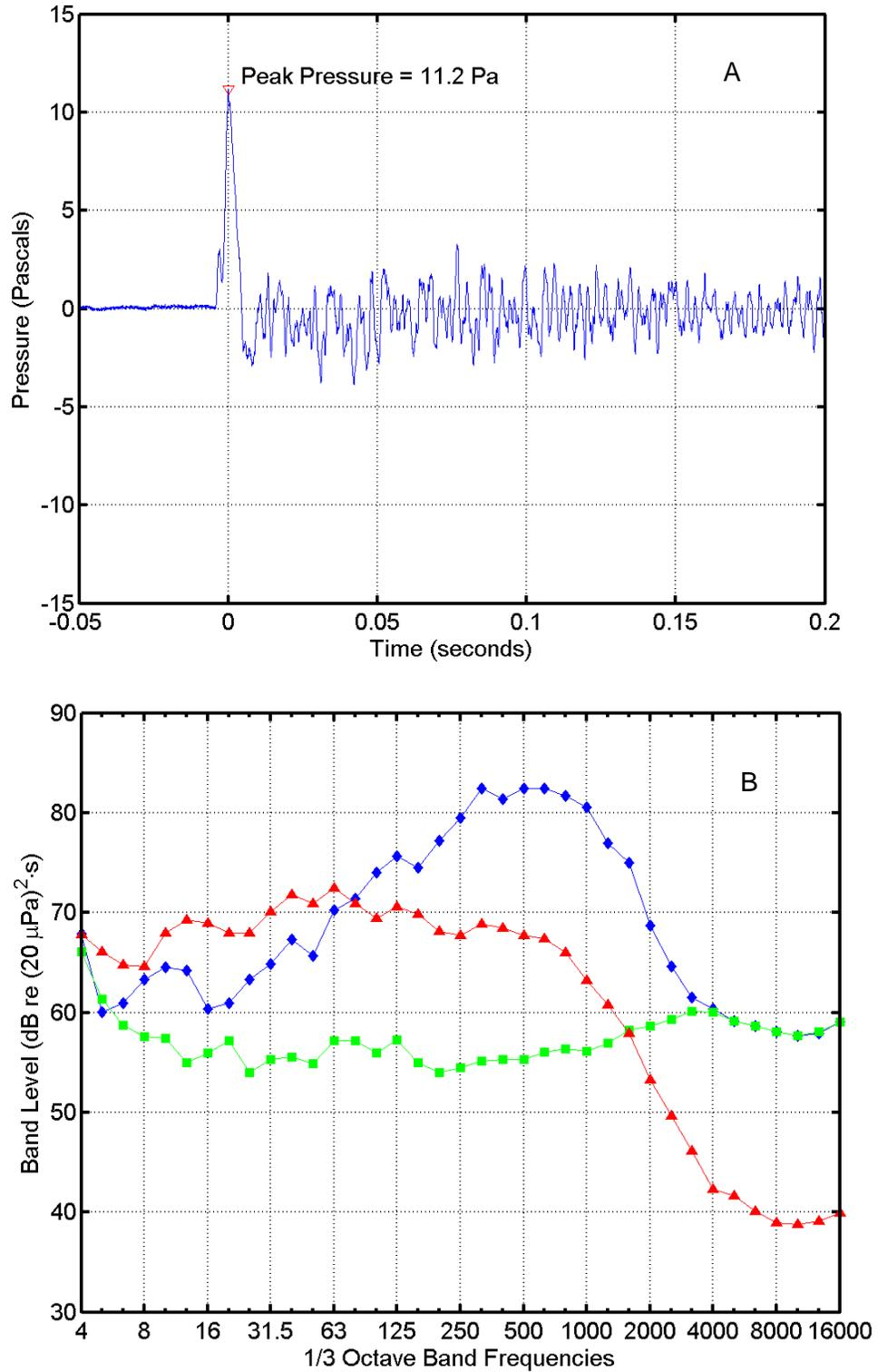
FIGURE C-6. (A) Pressure waveform and (B) one-third octave band levels for the second missile of the dual RAM launch at 11:46:12 on 5 May 2004 at "Bachelor Beach South". In (B),  $\diamond$  = missile sound energy;  $\square$  = instrumentation noise energy;  $\triangle$  = ambient noise power. Band frequencies in Hertz (Hz).
