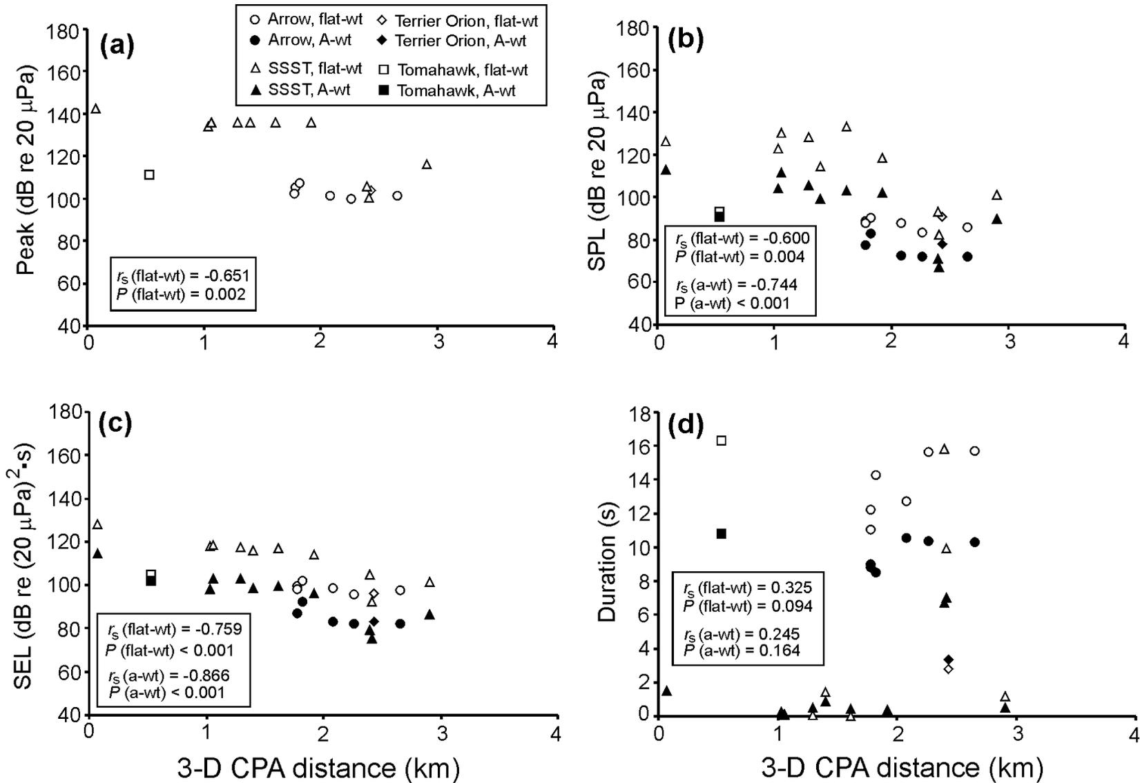
FIGURE 2.4. Sounds from other large vehicle (Terrier Orion, Tomahawk, Arrow, SSST) launches relative to the 3-D CPA distance: **(a)** Peak sound pressure, **(b)** SPL, **(c)** SEL, and **(d)** Duration. Plotted as in Figure 2.3.
