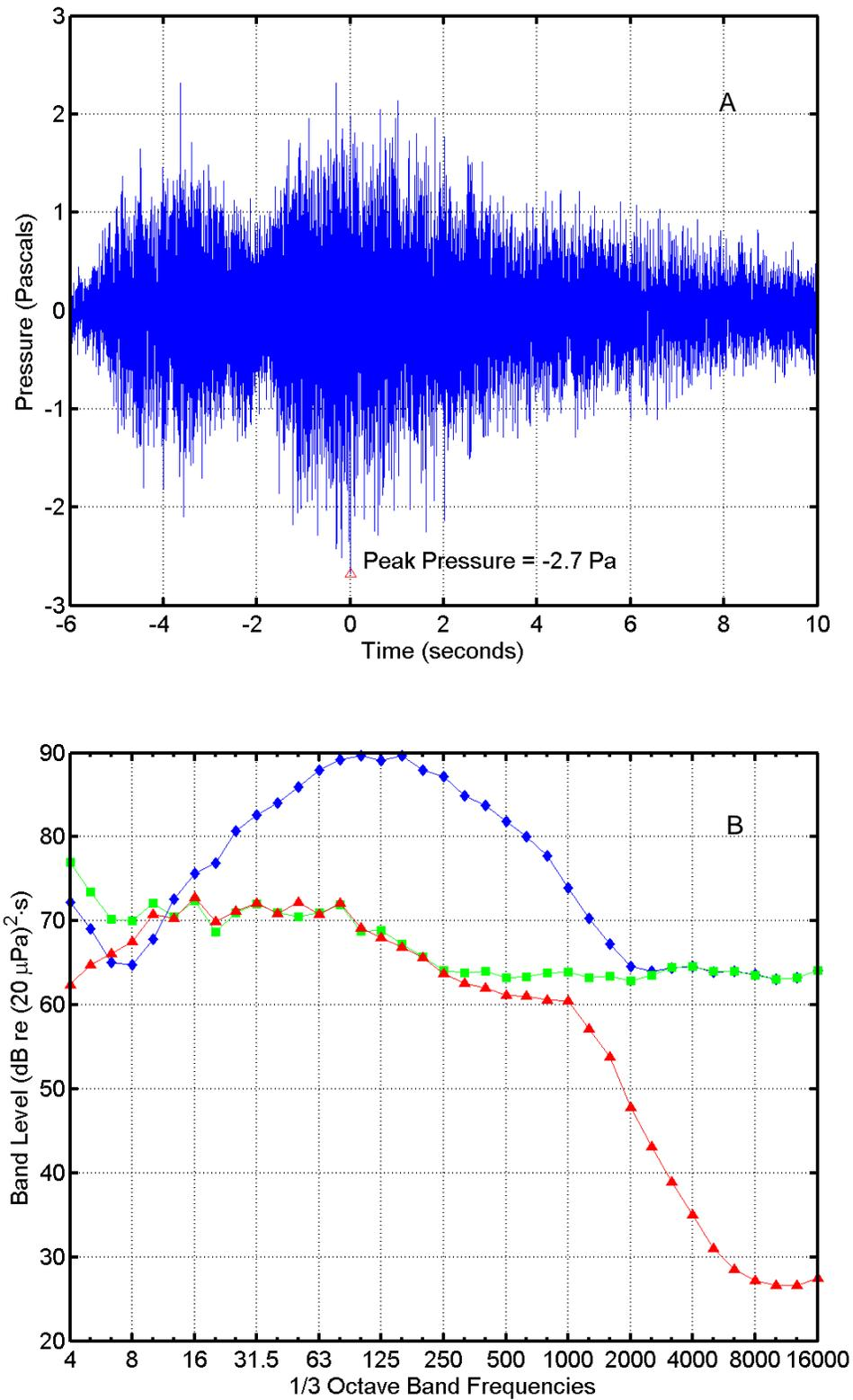
FIGURE C-28. (A) Pressure waveform and (B) one-third octave band levels for an Arrow flight at 10:08 on 26 August 2004 recorded "Dos Coves". In (B),  $\diamond$  = missile sound energy;  $\square$  = instrumentation noise energy;  $\Delta$  = ambient noise power. Band frequencies in Hertz (Hz).
