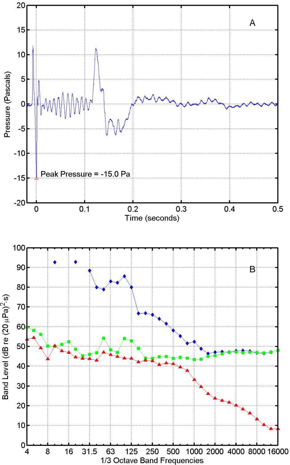
FIGURE C-12. (A) Pressure waveform and (B) one-third octave band levels for the AGS Slug launch at 11:31 on 3 June 2004 at "Dos Coves". In (B),  $\diamond$  = missile sound energy;  $\square$  = instrumentation noise energy;  $\Delta$  = ambient noise power. Band frequencies in Hertz (Hz).
