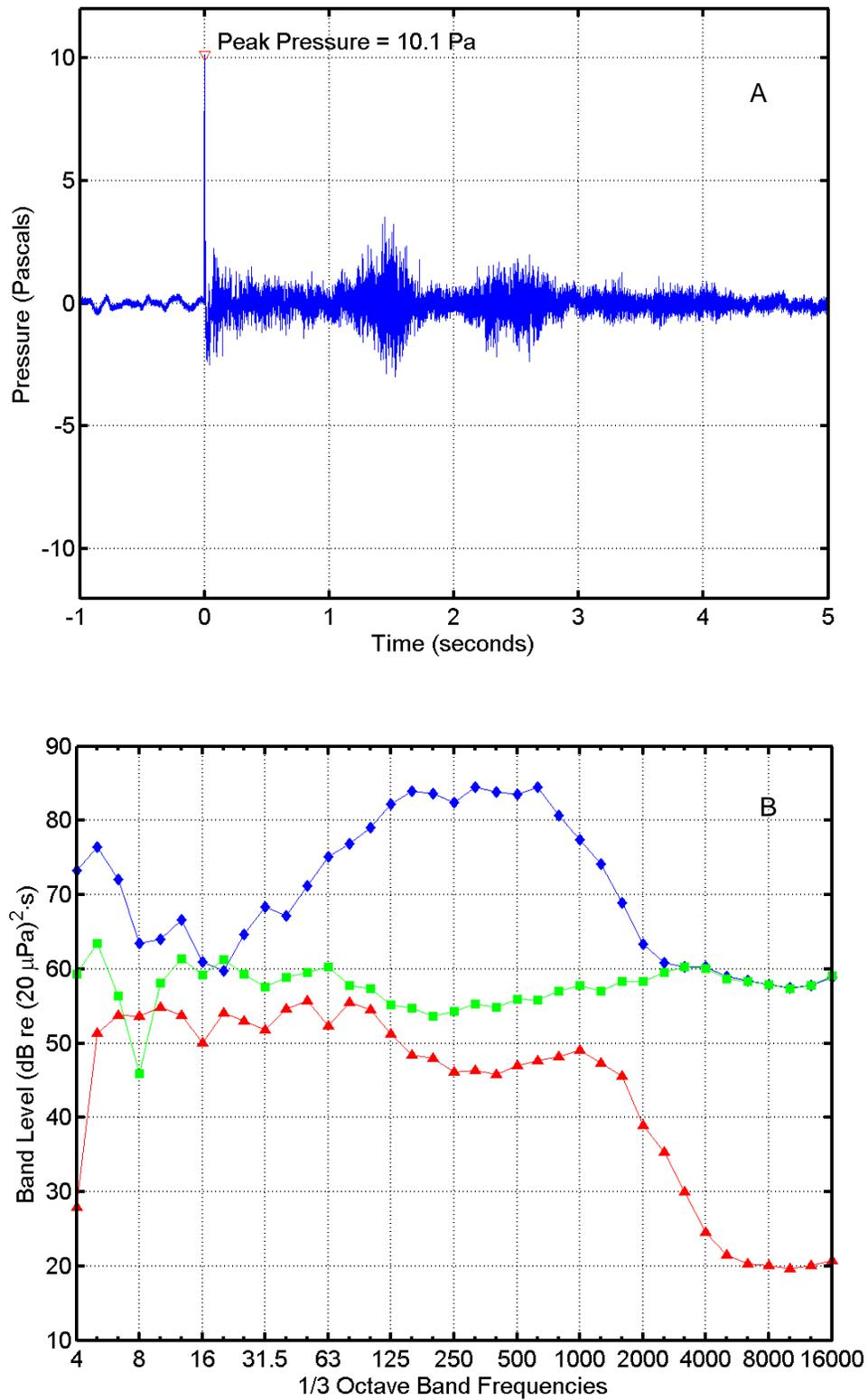
FIGURE C-40. (A) Pressure waveform and (B) one-third octave band levels for a RAM flight at 11:19 on 22 September 2004 recorded "Dos Coves South". In (B),  $\diamond$  = missile sound energy;  $\square$  = instrumentation noise energy;  $\Delta$  = ambient noise power. Band frequencies in Hertz (Hz).
