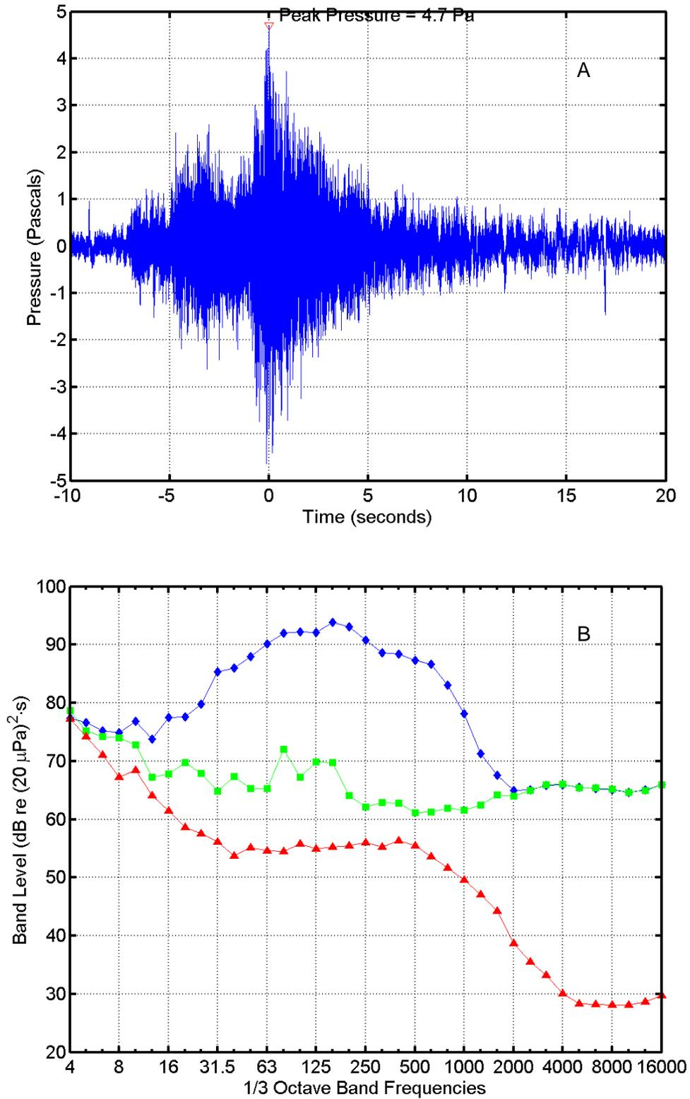
FIGURE C-26. (A) Pressure waveform and (B) one-third octave band levels for an Arrow flight at 10:20 on 29 July 2004 recorded "Bachelor Beach North". In (B),  $\diamond$  = missile sound energy;  $\square$  = instrumentation noise energy;  $\Delta$  = ambient noise power. Band frequencies in Hertz (Hz).
