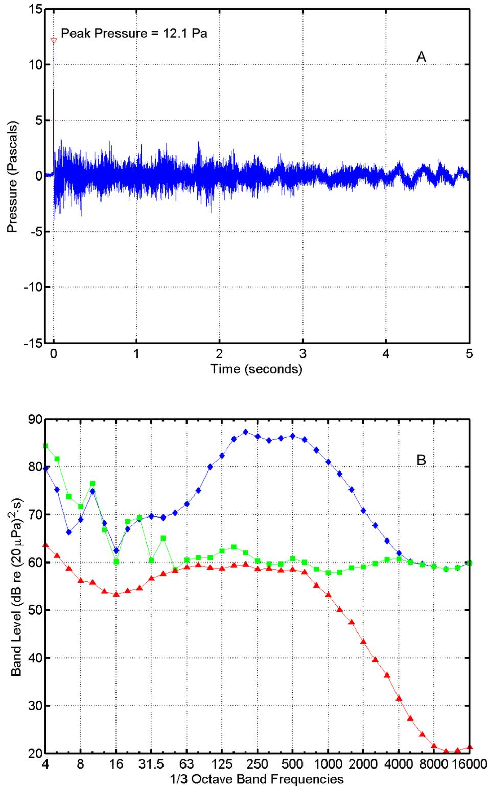
FIGURE C-3. (A) Pressure waveform and (B) one-third octave band levels for the first missile of the dual RAM launch at 11:46:00 on 5 May 2004 at "Bachelor Beach North". In (B),  $\diamond$  = missile sound energy;  $\square$  = instrumentation noise energy;  $\triangle$  = ambient noise power. Band frequencies in Hertz (Hz).
