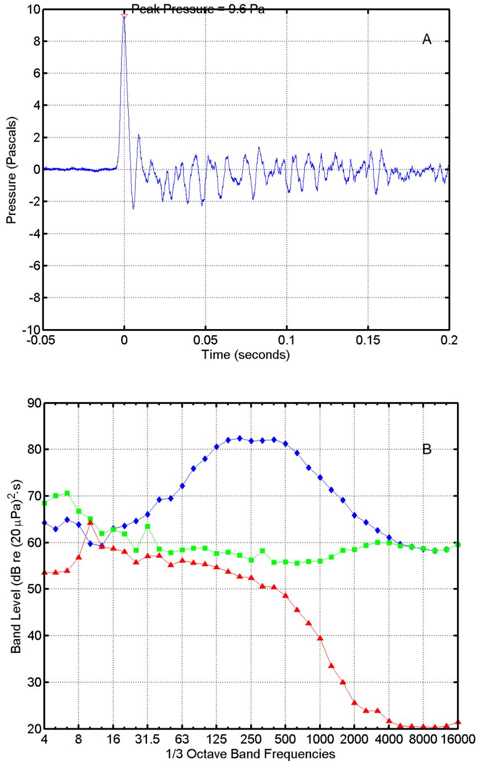
FIGURE C-2. (A) Pressure waveform and (B) one-third octave band levels for the second missile of the dual RAM launch at 11:46:12 on 5 May 2004 at "Dos Coves". In (B),  $\diamond$  = missile sound energy;  $\square$  = instrumentation noise energy;  $\triangle$  = ambient noise power. Band frequencies in Hertz (Hz).
