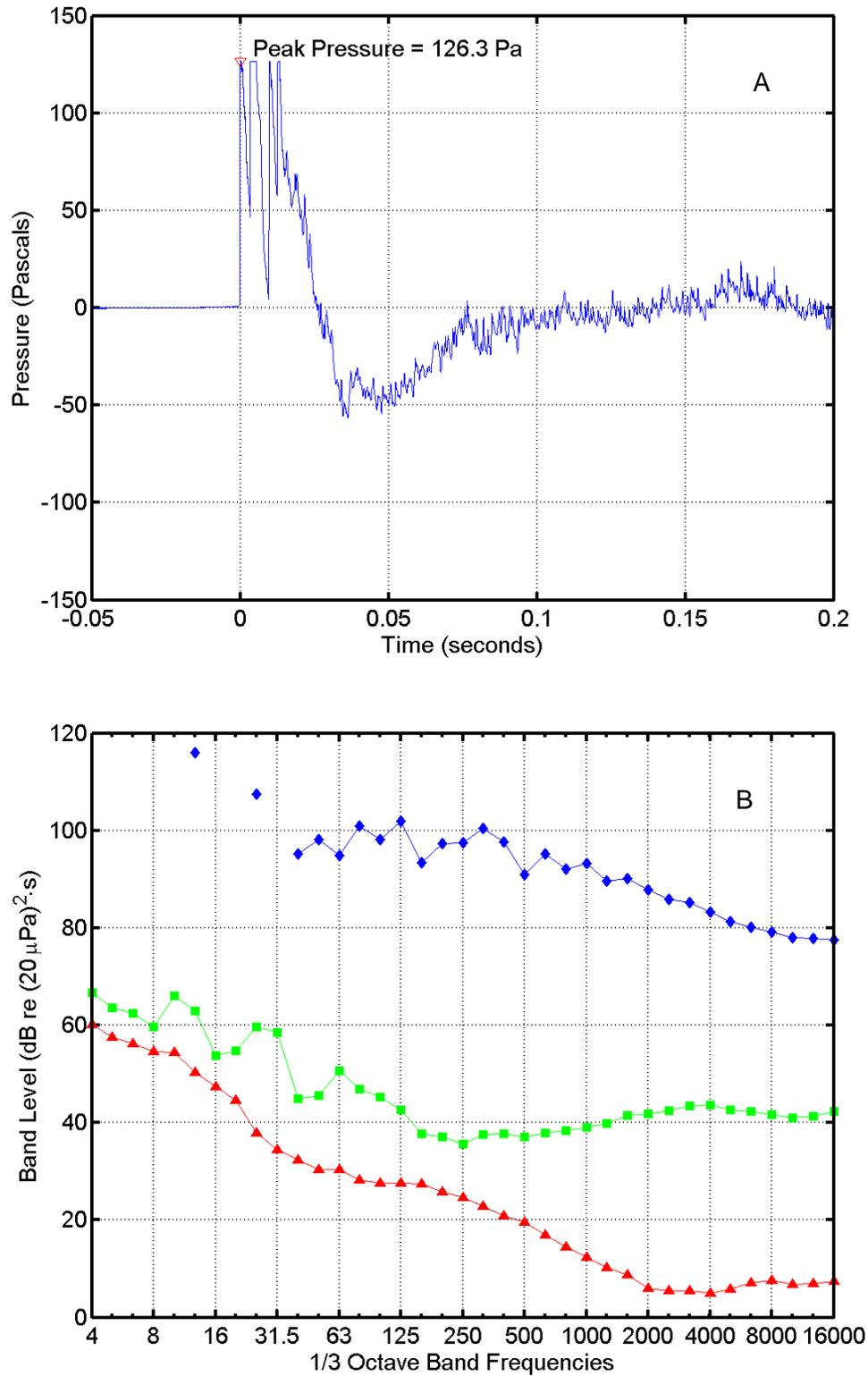
FIGURE C-7. (A) Pressure waveform and (B) one-third octave band levels for the SSST launch at 12:40 on 18 May 2004 at "Harbor Seal Overlook". In (B),  $\diamond$  = missile sound energy;  $\square$  = instrumentation noise energy;  $\Delta$  = ambient noise power. Band frequencies in Hertz (Hz).
