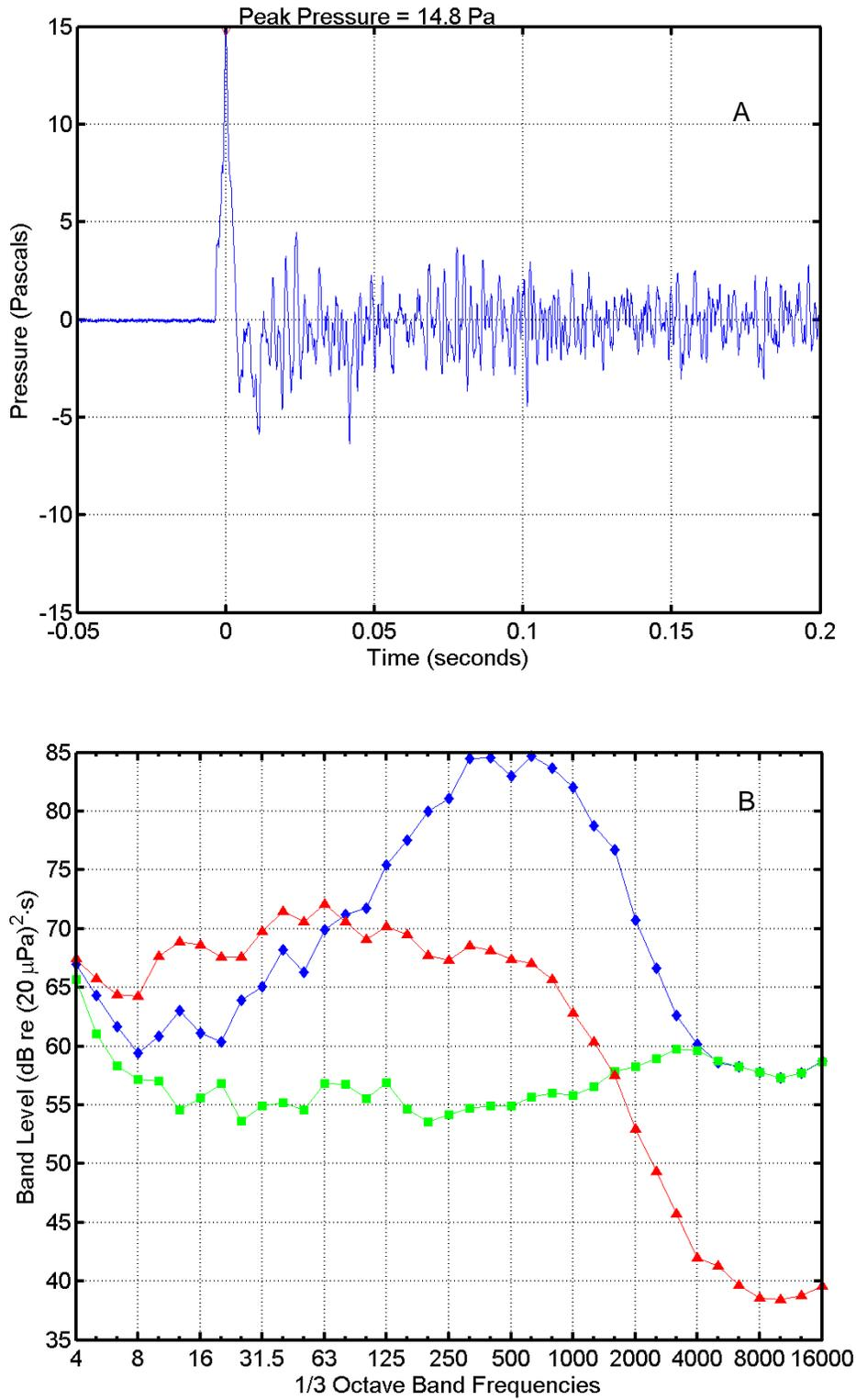
FIGURE C-5. (A) Pressure waveform and (B) one-third octave band levels for the first missile of the dual RAM launch at 11:46:00 on 5 May 2004 at "Bachelor Beach South". In (B),  $\diamond$  = missile sound energy;  $\square$  = instrumentation noise energy;  $\triangle$  = ambient noise power. Band frequencies in Hertz (Hz).
