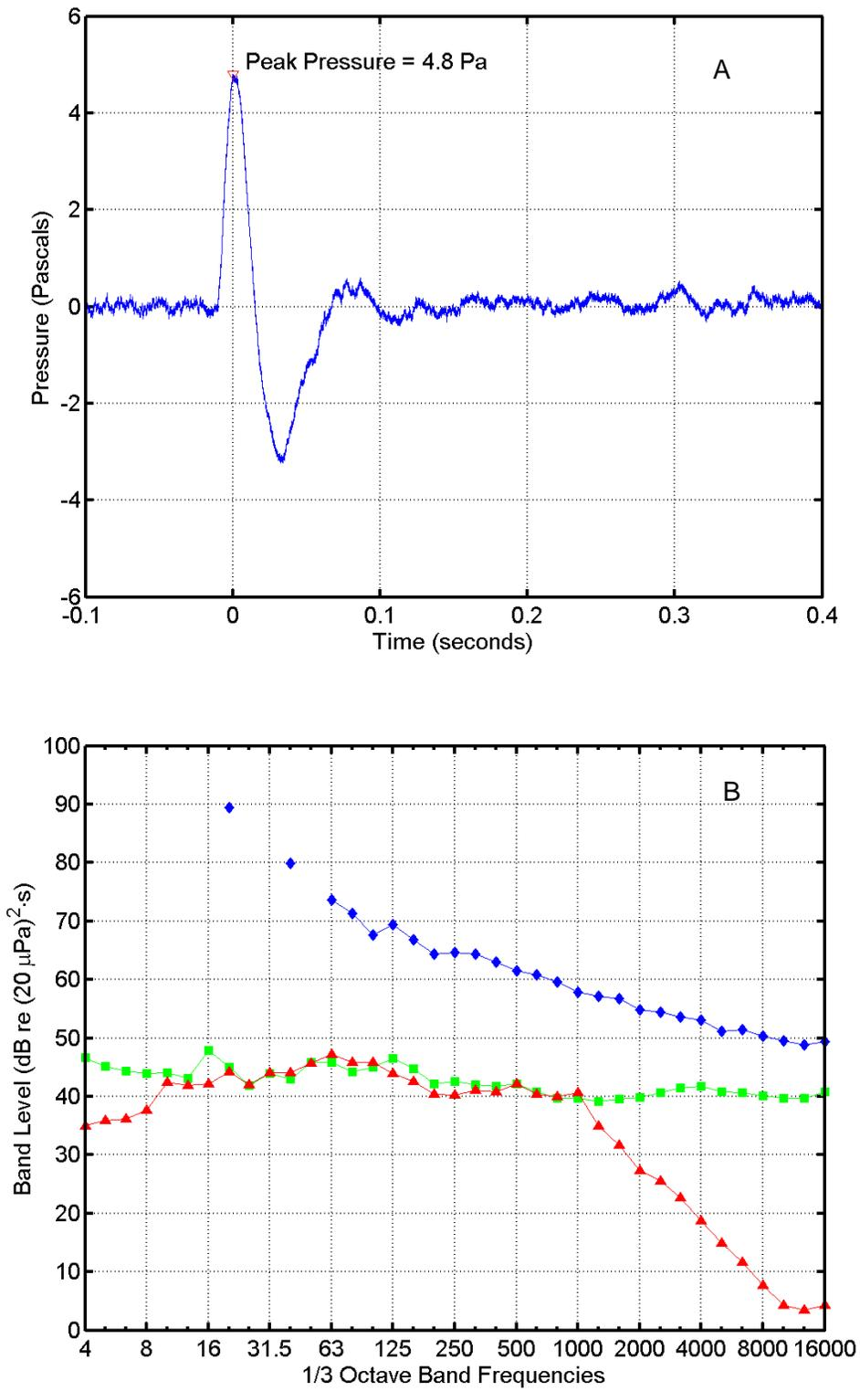
FIGURE C-48. (A) Pressure waveform and (B) one-third octave band levels for an AGS Missile flight at 13:29 on 27 January 2005 recorded at “Redeye I”. In (B),  $\diamond$  = missile sound energy;  $\square$  = instrumentation noise energy;  $\triangle$  = ambient noise power. Band frequencies in Hertz (Hz).
