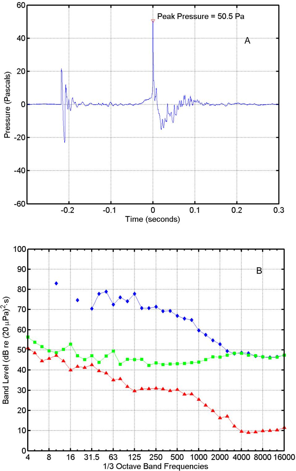
FIGURE C-13. (A) Pressure waveform and (B) one-third octave band levels for the AGS Slug launch at 13:22 on 3 June 2004 "Near 809 Camera". In (B),  $\diamond$  = missile sound energy;  $\square$  = instrumentation noise energy;  $\Delta$  = ambient noise power. Band frequencies in Hertz (Hz).
