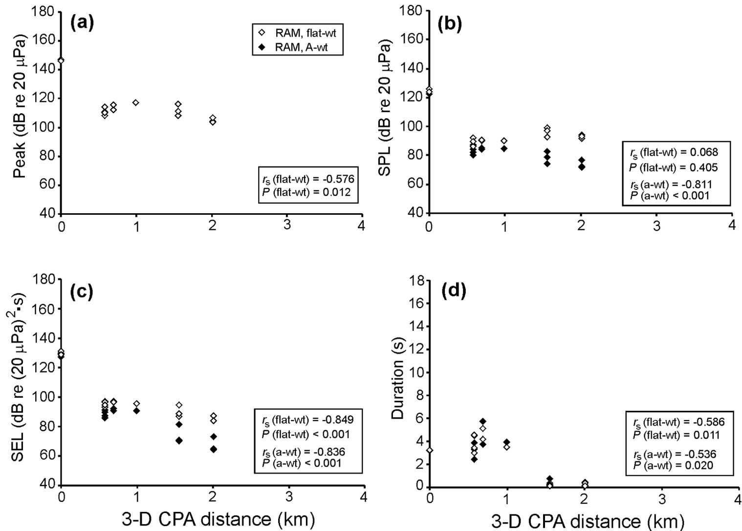
FIGURE 2.6. Sounds from launches of RAMs relative to the 3-D CPA distance: **(a)** Peak sound pressure, **(b)** SPL, **(c)** SEL, and **(d)** Duration. Plotted as in Figure 2.3.
