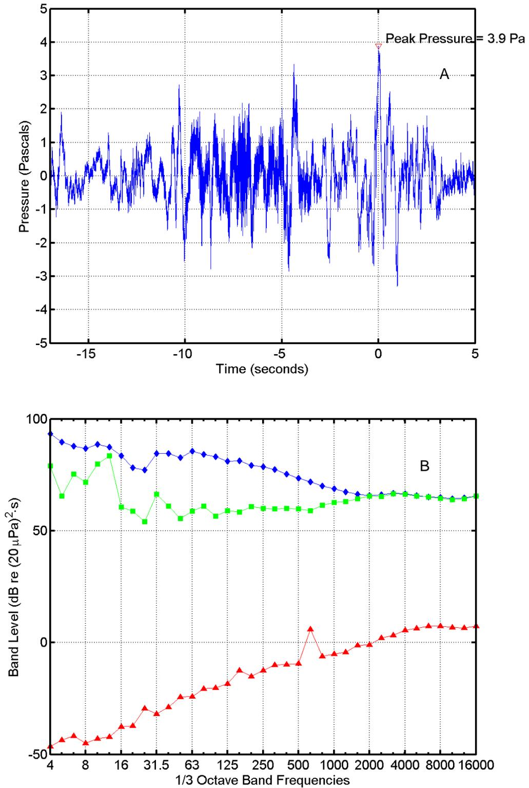
FIGURE C-8. (A) Pressure waveform and (B) one-third octave band levels for the SSST launch at 12:40 on 18 May 2004 at "Pirates Cove". In (B),  $\diamond$  = missile sound energy;  $\square$  = instrumentation noise energy;  $\triangle$  = ambient noise power. Band frequencies in Hertz (Hz).
