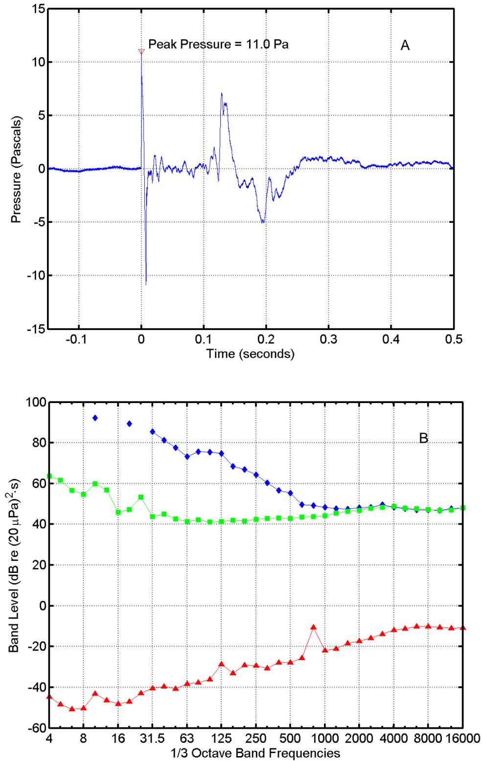
FIGURE C-14. (A) Pressure waveform and (B) one-third octave band levels for the AGS Slug launch at 13:22 on 3 June 2004 at “Harbor Seal Overlook”. In (B),  $\diamond$  = missile sound energy;  $\square$  = instrumentation noise energy;  $\triangle$  = ambient noise power. Band frequencies in Hertz (Hz).
