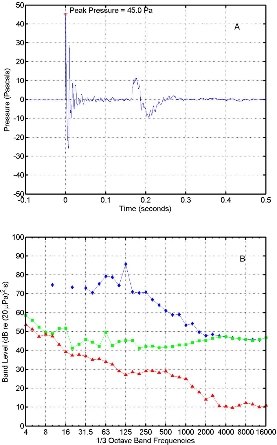
FIGURE C-10. (A) Pressure waveform and (B) one-third octave band levels for the AGS Slug launch at 11:31 on 3 June 2004 “Near 809 Camera”. In (B),  $\diamond$  = missile sound energy;  $\square$  = instrumentation noise energy;  $\Delta$  = ambient noise power. Band frequencies in Hertz (Hz).
