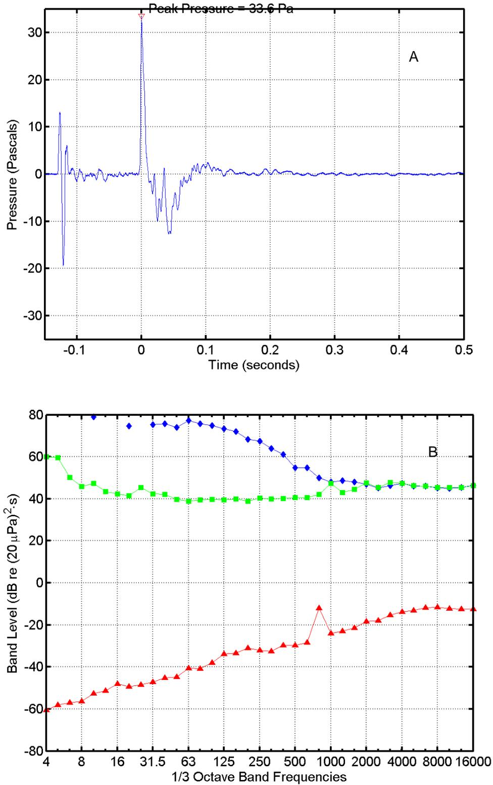
FIGURE C-11. (A) Pressure waveform and (B) one-third octave band levels for the AGS Slug launch at 11:31 on 3 June 2004 at "Harbor Seal Overlook". In (B),  $\diamond$  = missile sound energy;  $\square$  = instrumentation noise energy;  $\triangle$  = ambient noise power. Band frequencies in Hertz (Hz).
