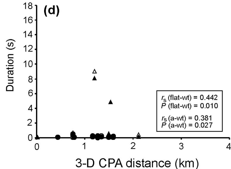
FIGURE 2.5. Sounds from launches of AGS vehicles relative to the 3-D CPA distance: **(a)** Peak sound pressure, **(b)** SPL, **(c)** SEL, and **(d)** Duration. Plotted as in Figure 2.3.
