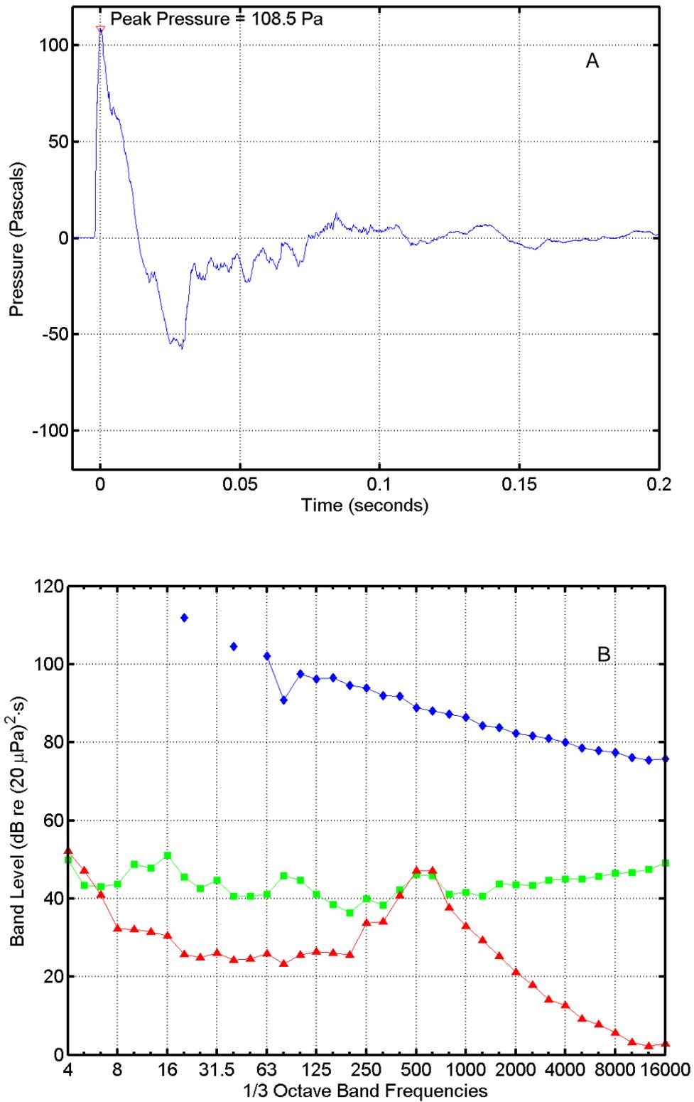
FIGURE C-24. (A) Pressure waveform and (B) one-third octave band levels for the AGS Slug launch at 15:43 on 26 July 2004 at "Dos Coves South". In (B),  $\diamond$  = missile sound energy;  $\square$  = instrumentation noise energy;  $\Delta$  = ambient noise power. Band frequencies in Hertz (Hz).
