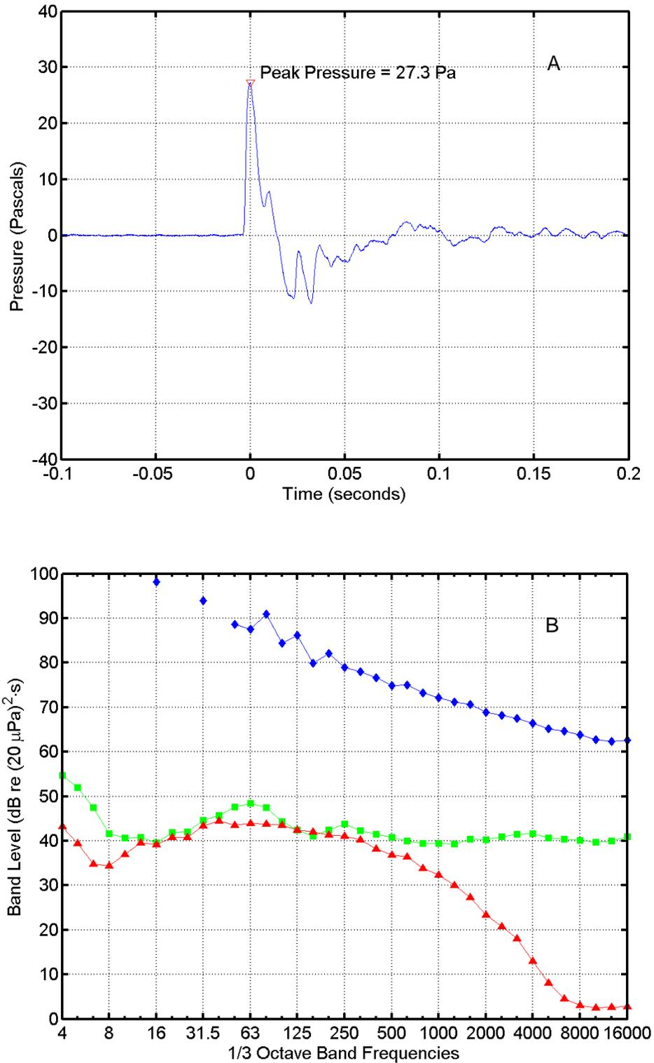
FIGURE C-45. (A) Pressure waveform and (B) one-third octave band levels for an AGS Slug flight at 11:41 on 27 January 2005 recorded at "Bachelor Beach North". In (B),  $\diamond$  = missile sound energy;  $\square$  = instrumentation noise energy;  $\Delta$  = ambient noise power. Band frequencies in Hertz (Hz).
