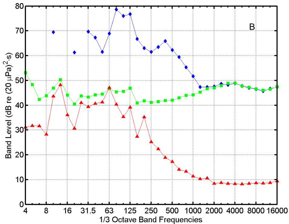
FIGURE C-39. (A) Pressure waveform and (B) one-third octave band levels for a RAM flight at 10:57 on 22 September 2004 recorded “The Y”. In (B),  $\diamond$  = missile sound energy;  $\square$  = instrumentation noise energy;  $\Delta$  = ambient noise power. Band frequencies in Hertz (Hz).
