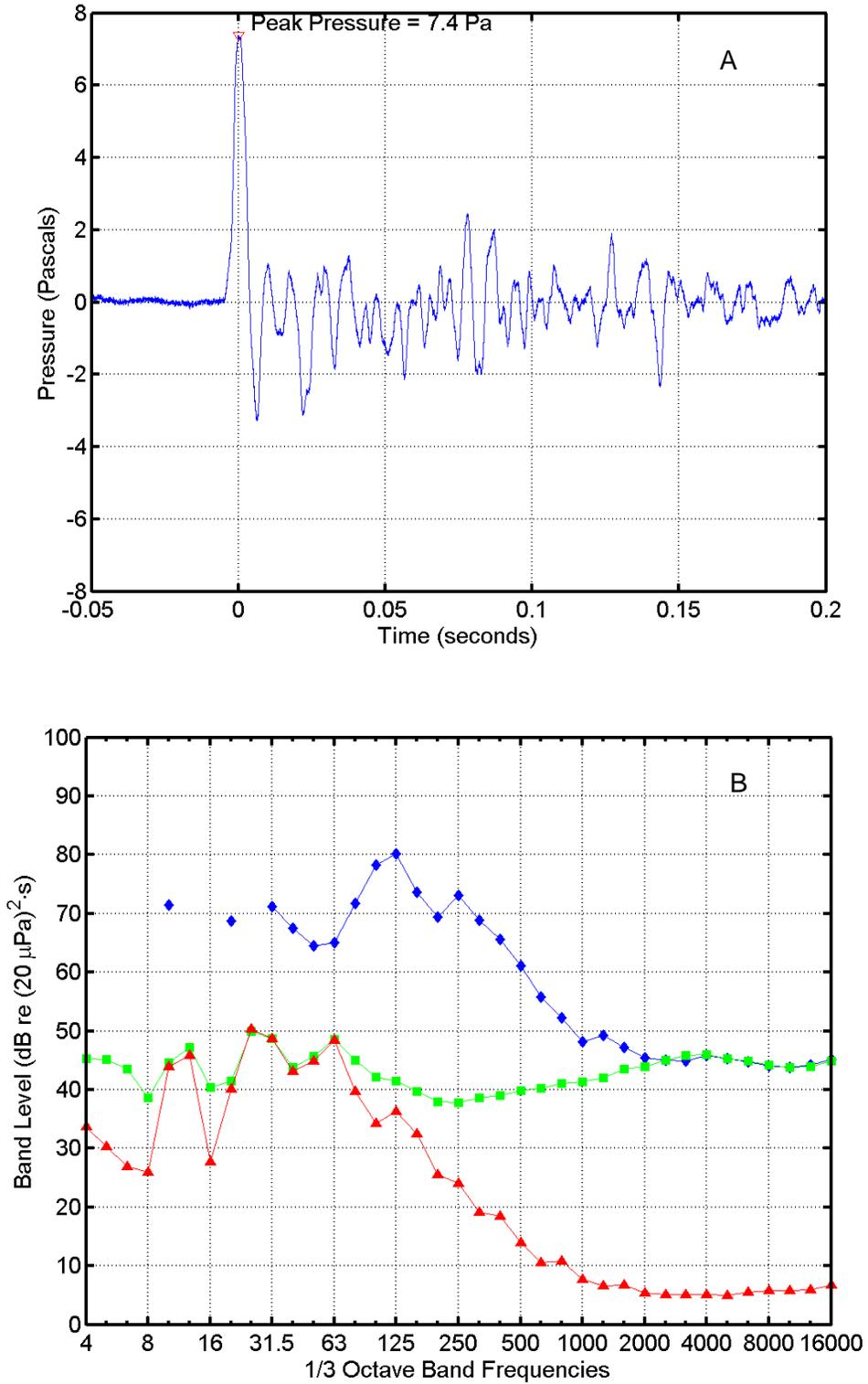
FIGURE C-42. (A) Pressure waveform and (B) one-third octave band levels for a RAM flight at 11:19 on 22 September 2004 recorded “The Y”. In (B),  $\diamond$  = missile sound energy;  $\square$  = instrumentation noise energy;  $\Delta$  = ambient noise power. Band frequencies in Hertz (Hz).
