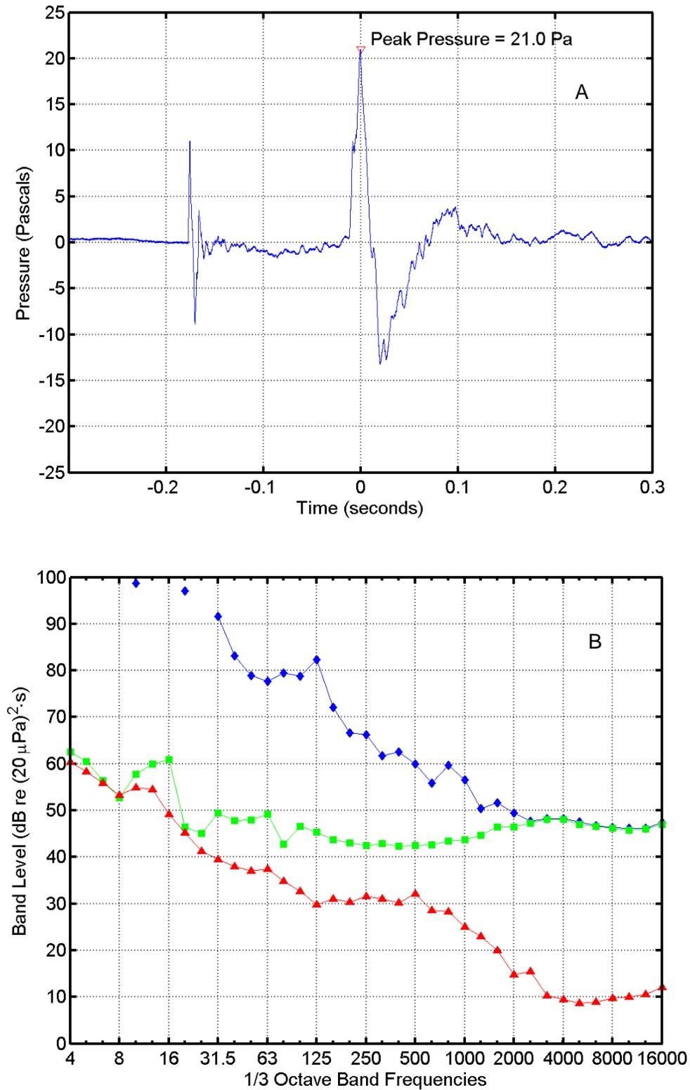
FIGURE C-16. (A) Pressure waveform and (B) one-third octave band levels for the AGS Missile launch at 15:08 on 3 June 2004 "Near 809 Camera". In (B),  $\diamond$  = missile sound energy;  $\square$  = instrumentation noise energy;  $\Delta$  = ambient noise power. Band frequencies in Hertz (Hz).
