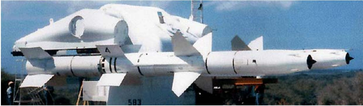
FIGURE 1.4. View of two Vandals mounted on the launch pad at the Alpha Complex on San Nicolas Island; solid rocket booster is visible at rear of closer Vandal (photograph by U.S. Navy).
