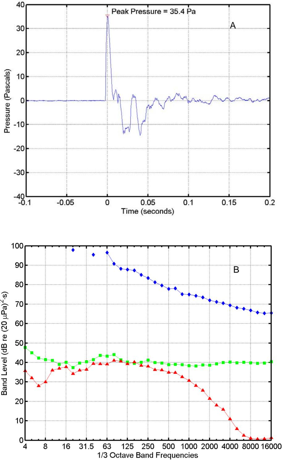
FIGURE C-43. (A) Pressure waveform and (B) one-third octave band levels for an AGS Slug flight at 8:59 on 27 January 2005 recorded at "Bachelor Beach North". In (B),  $\diamond$  = missile sound energy;  $\square$  = instrumentation noise energy;  $\Delta$  = ambient noise power. Band frequencies in Hertz (Hz).
