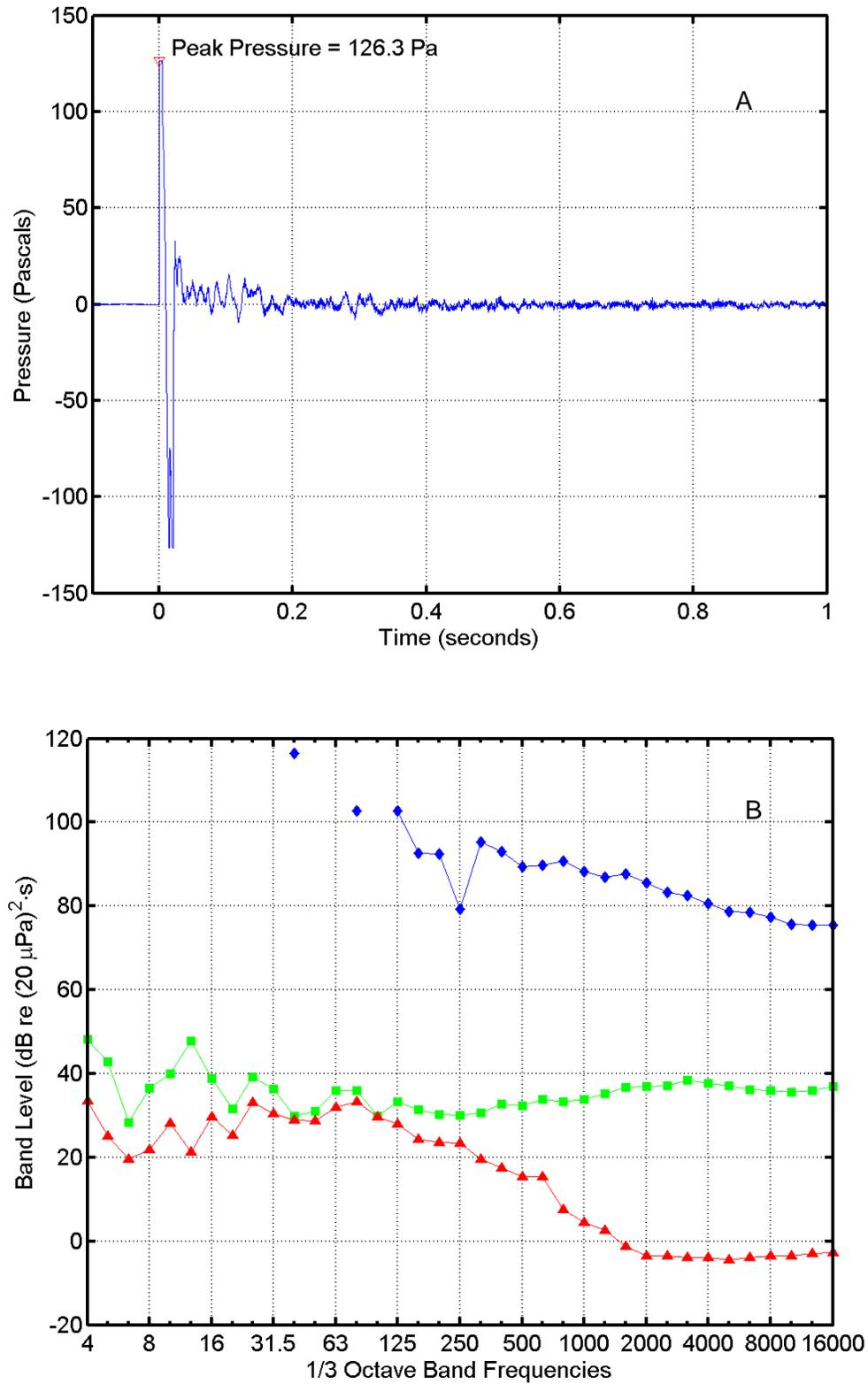
FIGURE C-33. (A) Pressure waveform and (B) one-third octave band levels for the SSST launch at 16:30 on 27 August 2004 recorded "Vizcaino Point". In (B),  $\diamond$  = missile sound energy;  $\square$  = instrumentation noise energy;  $\Delta$  = ambient noise power. Band frequencies in Hertz (Hz).
