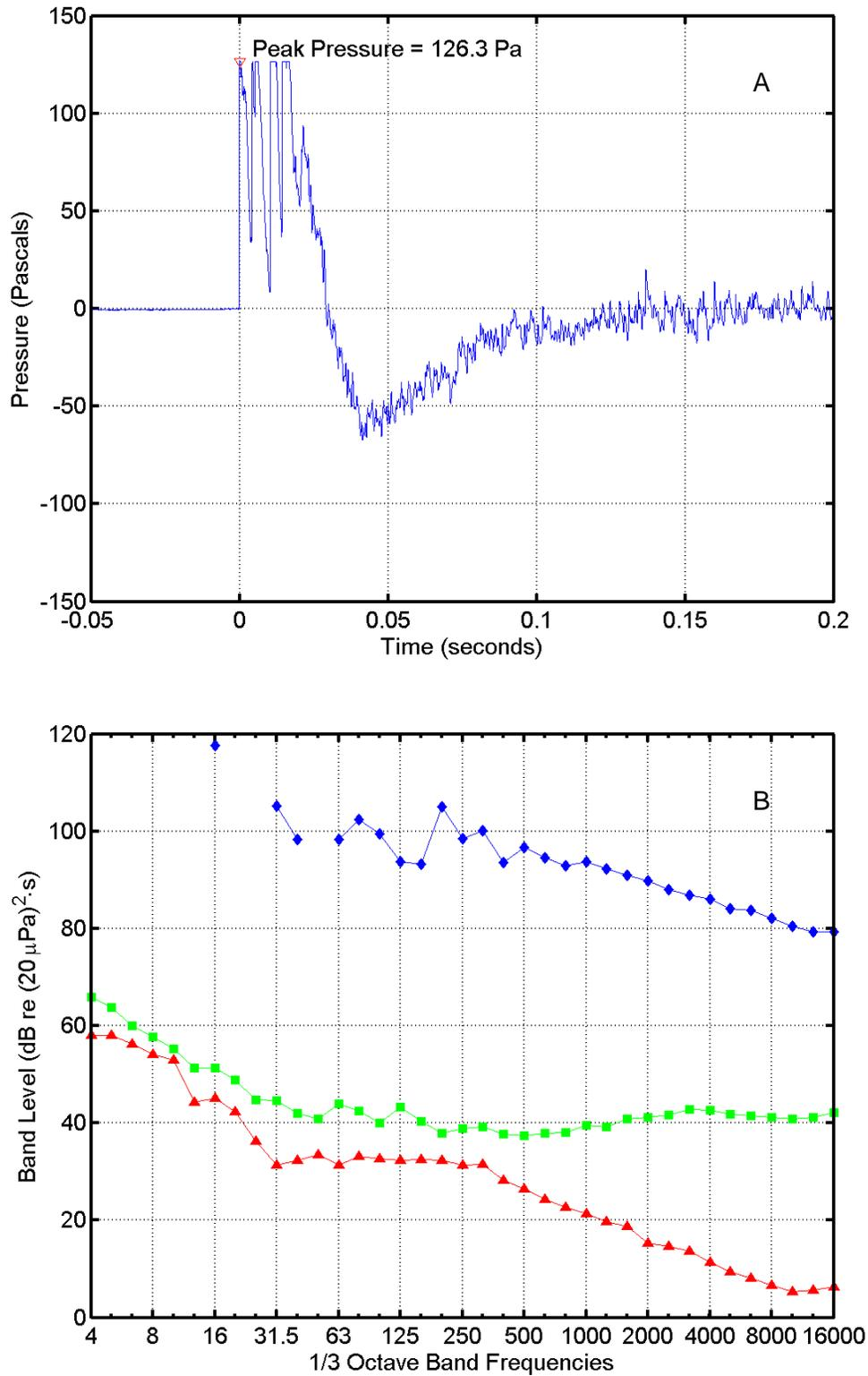
FIGURE C-9. (A) Pressure waveform and (B) one-third octave band levels for the SSST launch at 12:40 on 18 May 2004 at "Redeye I". In (B),  $\diamond$  = missile sound energy;  $\square$  = instrumentation noise energy;  $\Delta$  = ambient noise power. Band frequencies in Hertz (Hz).
