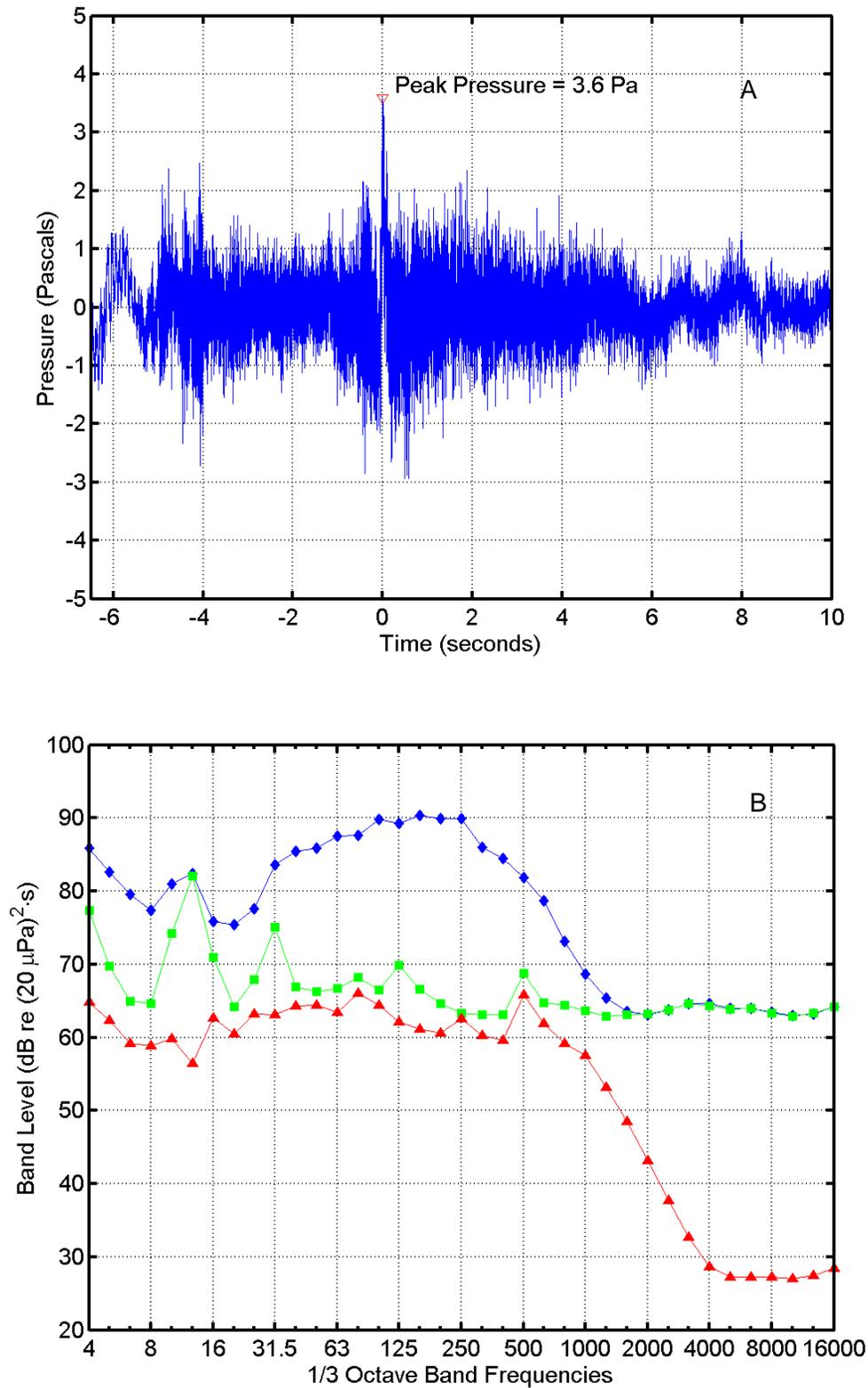
FIGURE C-27. (A) Pressure waveform and (B) one-third octave band levels for an Arrow flight at 10:20 on 29 July 2004 recorded "Dos Coves South". In (B),  $\diamond$  = missile sound energy;  $\square$  = instrumentation noise energy;  $\Delta$  = ambient noise power. Band frequencies in Hertz (Hz).
