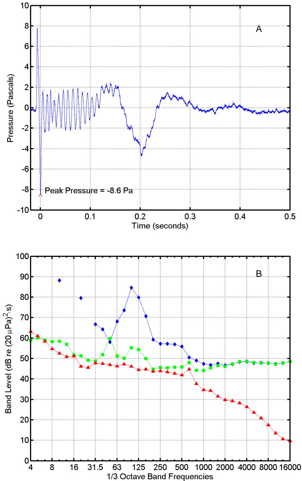
FIGURE C-15. (A) Pressure waveform and (B) one-third octave band levels for the AGS Slug launch at 13:22 on 3 June 2004 at "Dos Coves". In (B),  $\diamond$  = missile sound energy;  $\square$  = instrumentation noise energy;  $\Delta$  = ambient noise power. Band frequencies in Hertz (Hz).
