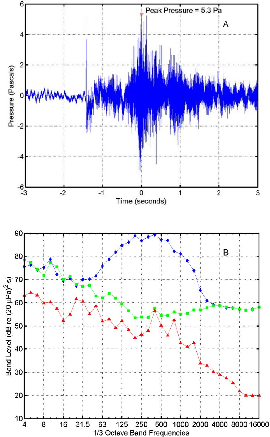
FIGURE C-34. (A) Pressure waveform and (B) one-third octave band levels for a RAM flight at 9:56 on 22 September 2004 recorded "Dos Coves South". In (B),  $\diamond$  = missile sound energy;  $\square$  = instrumentation noise energy;  $\triangle$  = ambient noise power. Band frequencies in Hertz (Hz).
