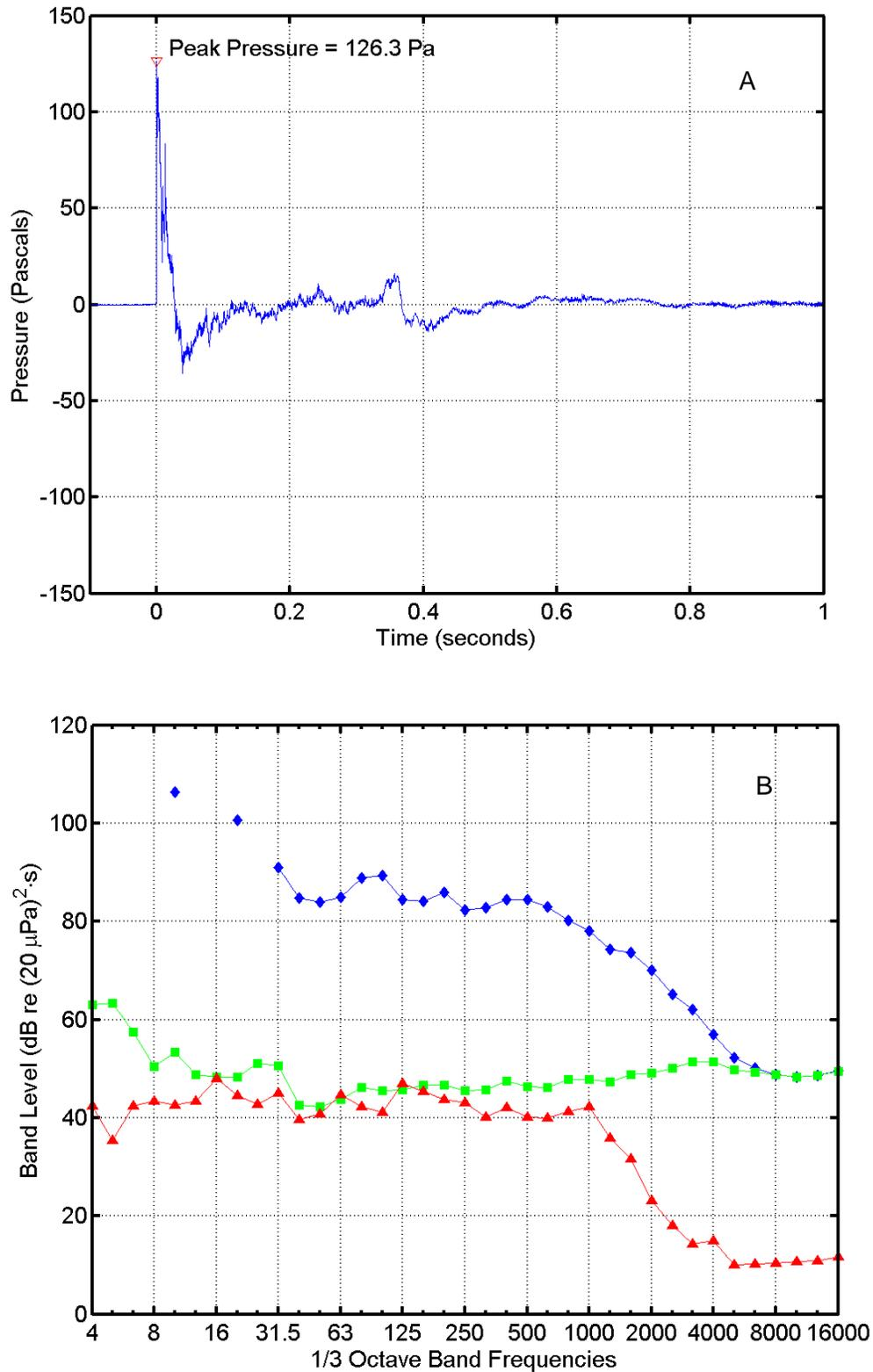
FIGURE C-31. (A) Pressure waveform and (B) one-third octave band levels for a SSST launch at 16:30 on 27 August 2004 recorded “Dos Coves”. In (B),  $\diamond$  = missile sound energy;  $\square$  = instrumentation noise energy;  $\Delta$  = ambient noise power. Band frequencies in Hertz (Hz).
