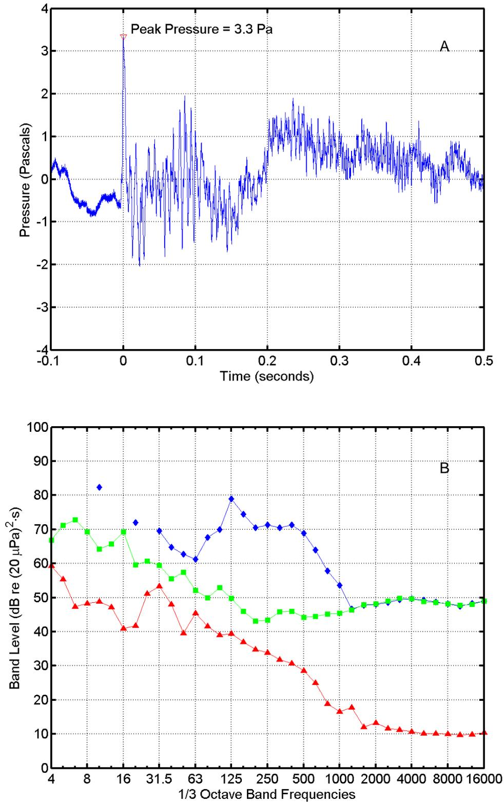
FIGURE C-35. (A) Pressure waveform and (B) one-third octave band levels for a RAM flight at 9:56 on 22 September 2004 recorded "Vizcaino Point". In (B),  $\diamond$  = missile sound energy;  $\square$  = instrumentation noise energy;  $\Delta$  = ambient noise power. Band frequencies in Hertz (Hz).
