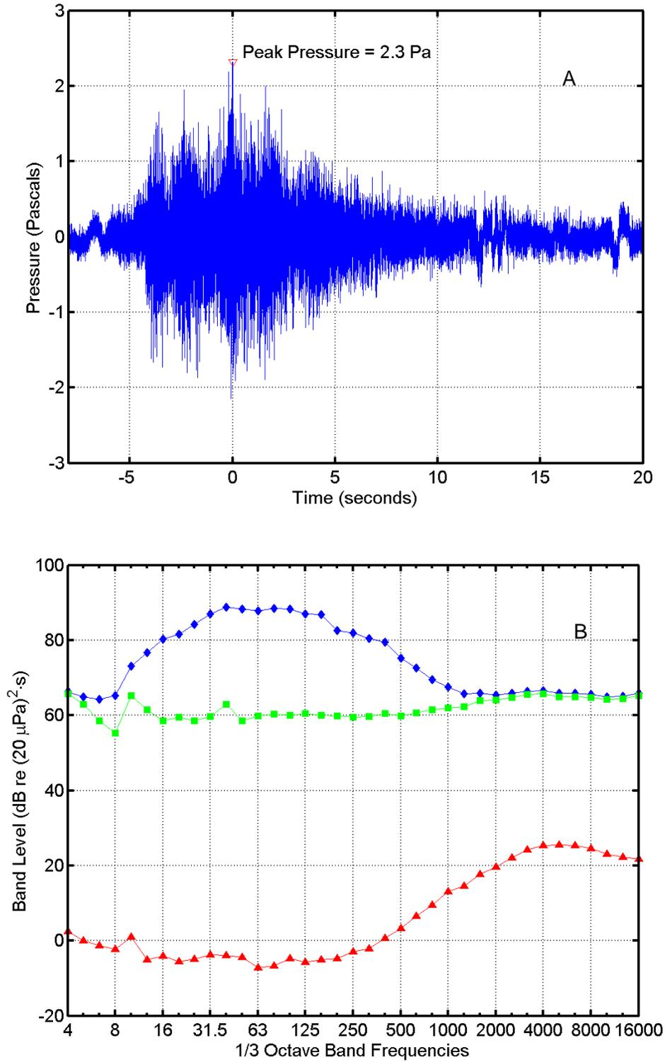
FIGURE C-29. (A) Pressure waveform and (B) one-third octave band levels for an Arrow flight at 10:08 on 26 August 2004 recorded "Phoca Reef". In (B),  $\diamond$  = missile sound energy;  $\square$  = instrumentation noise energy;  $\Delta$  = ambient noise power. Band frequencies in Hertz (Hz).
