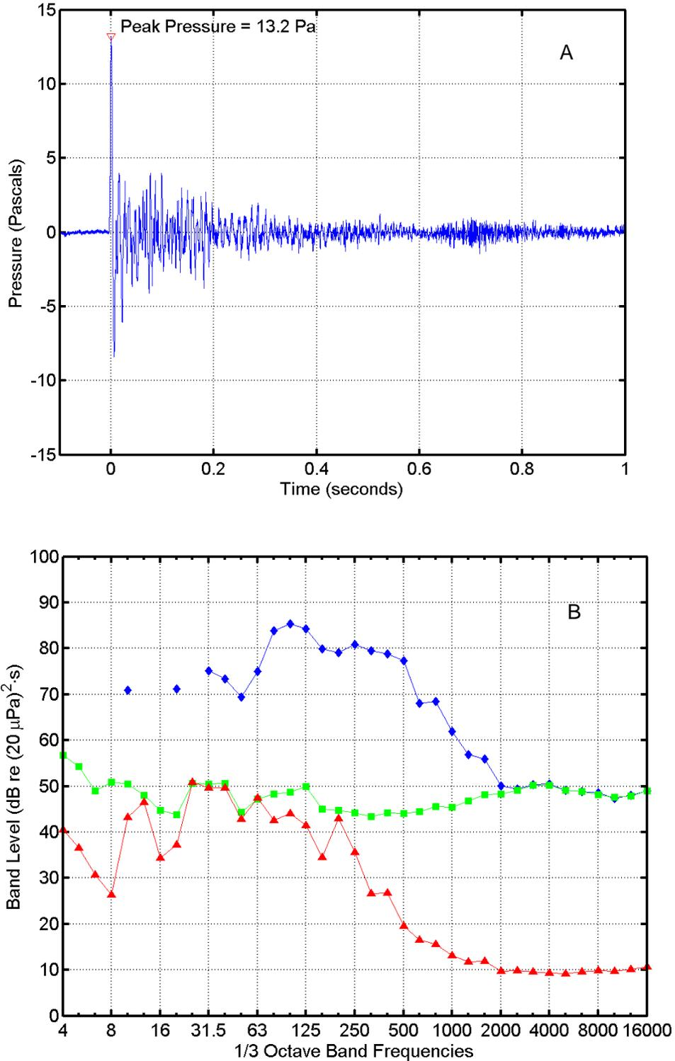
FIGURE C-36. (A) Pressure waveform and (B) one-third octave band levels for a RAM flight at 9:56 on 22 September 2004 recorded "The Y". In (B),  $\diamond$  = missile sound energy;  $\square$  = instrumentation noise energy;  $\triangle$  = ambient noise power. Band frequencies in Hertz (Hz).
