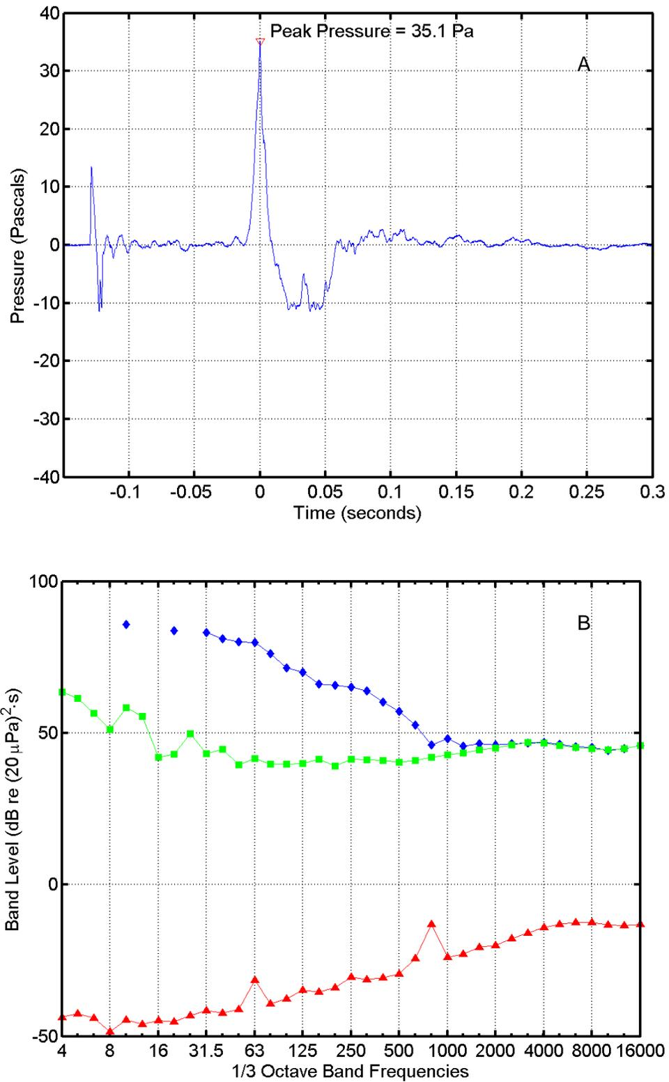
FIGURE C-17. (A) Pressure waveform and (B) one-third octave band levels for the AGS Missile launch at 15:08 on 3 June 2004 at "Harbor Seal Overlook". In (B),  $\diamond$  = missile sound energy;  $\square$  = instrumentation noise energy;  $\triangle$  = ambient noise power. Band frequencies in Hertz (Hz).
