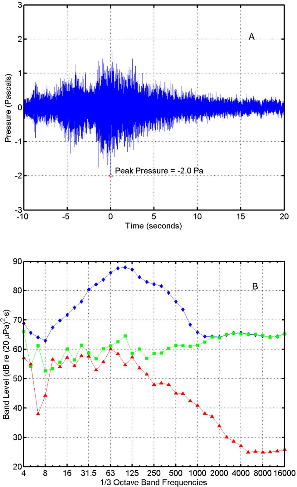
FIGURE C-30. (A) Pressure waveform and (B) one-third octave band levels for an Arrow flight at 10:08 on 26 August 2004 recorded "Vizcaino Point". In (B),  $\diamond$  = missile sound energy;  $\square$  = instrumentation noise energy;  $\Delta$  = ambient noise power. Band frequencies in Hertz (Hz).
