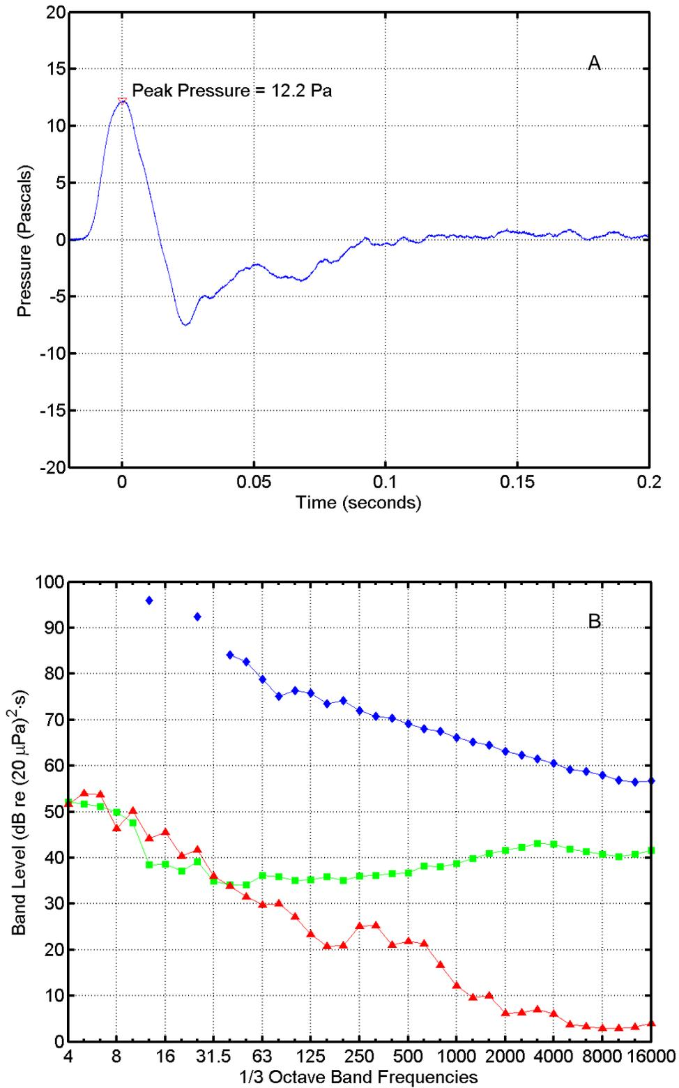
FIGURE C-23. (A) Pressure waveform and (B) one-third octave band levels for the AGS Slug launch at 15:43 on 26 July 2004 at "Vizcaino Point". In (B),  $\diamond$  = missile sound energy;  $\square$  = instrumentation noise energy;  $\Delta$  = ambient noise power. Band frequencies in Hertz (Hz).
