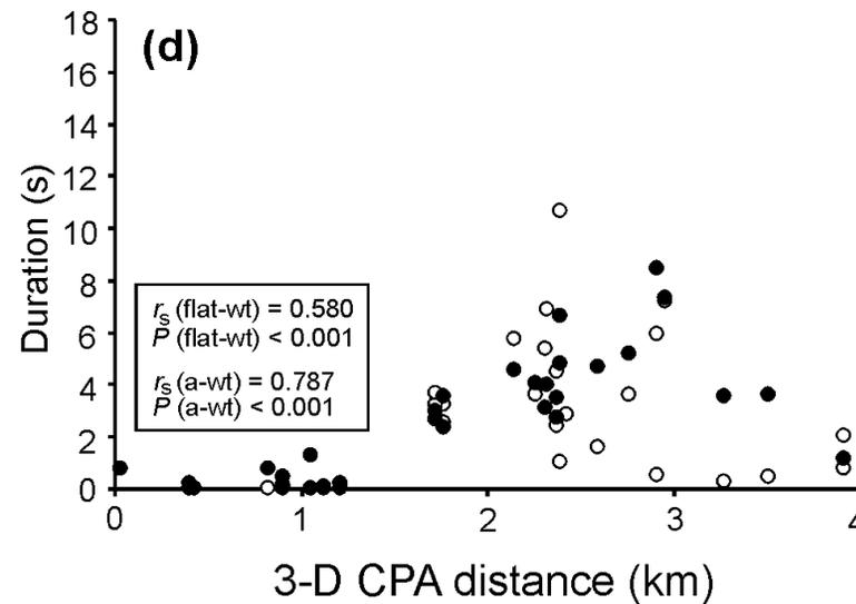
FIGURE 2.3. Sounds from launches of Vandal missiles relative to the 3-D CPA distance: **(a)** Peak sound pressure, **(b)** SPL, **(c)** SEL, and **(d)** Duration. For SPL, SEL, and Duration, both flat-weighted (open symbols) and A-weighted (closed symbols) measurements are shown. Also shown are Spearman rank order correlation coefficients ( $r_s$ ) along with 1-sided  $P$ -values.
