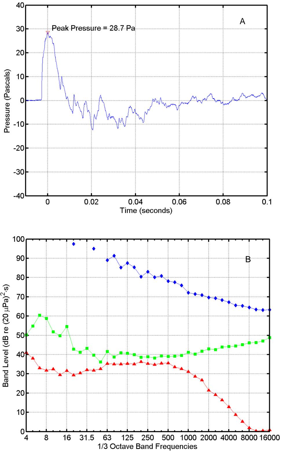
FIGURE C-19. (A) Pressure waveform and (B) one-third octave band levels for the AGS Slug launch at 15:10 on 26 July 2004 at "Bachelor Beach North". In (B),  $\diamond$  = missile sound energy;  $\square$  = instrumentation noise energy;  $\triangle$  = ambient noise power. Band frequencies in Hertz (Hz).
