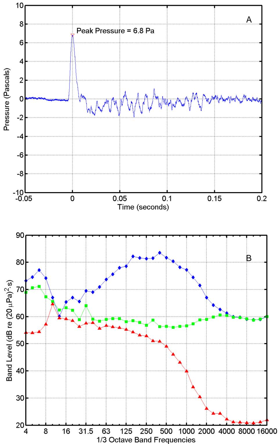
FIGURE C-1. (A) Pressure waveform and (B) one-third octave band levels for the first missile of the dual RAM launch at 11:46:00 on 5 May 2004 at "Dos Coves". In (B),  $\diamond$  = missile sound energy;  $\square$  = instrumentation noise energy;  $\triangle$  = ambient noise power. Band frequencies in Hertz (Hz).
