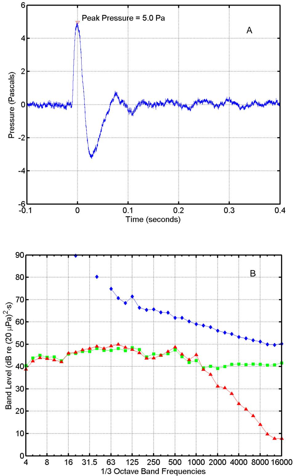
FIGURE C-44. (A) Pressure waveform and (B) one-third octave band levels for an AGS Slug flight at 8:59 on 27 January 2005 recorded at "Redeye I". In (B),  $\diamond$  = missile sound energy;  $\square$  = instrumentation noise energy;  $\Delta$  = ambient noise power. Band frequencies in Hertz (Hz).
