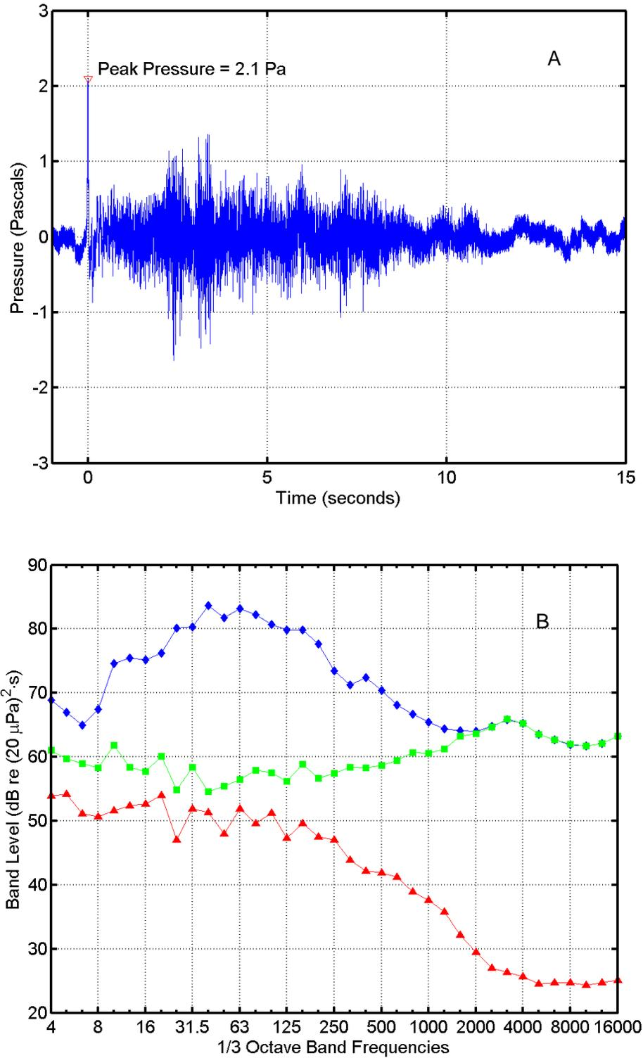
FIGURE C-32. (A) Pressure waveform and (B) one-third octave band levels for the SSST launch at 16:30 on 27 August 2004 recorded "Phoca Reef". In (B),  $\diamond$  = missile sound energy;  $\square$  = instrumentation noise energy;  $\Delta$  = ambient noise power. Band frequencies in Hertz (Hz).
