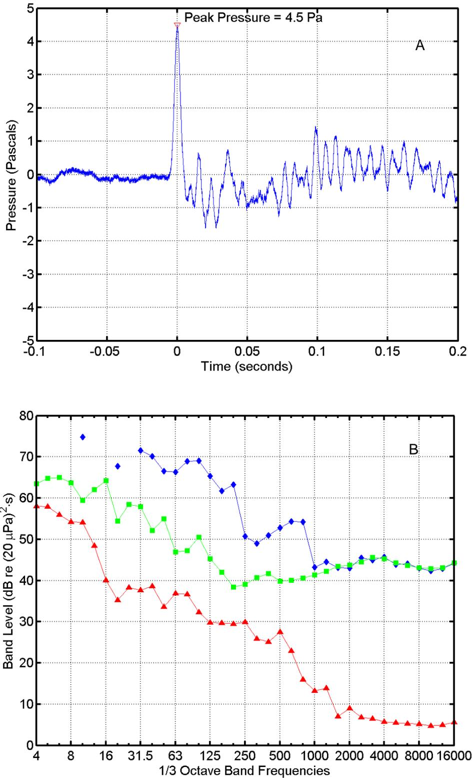
FIGURE C-41. (A) Pressure waveform and (B) one-third octave band levels for a RAM flight at 11:19 on 22 September 2004 recorded "Vizcaino Point". In (B),  $\diamond$  = missile sound energy;  $\square$  = instrumentation noise energy;  $\Delta$  = ambient noise power. Band frequencies in Hertz (Hz).
