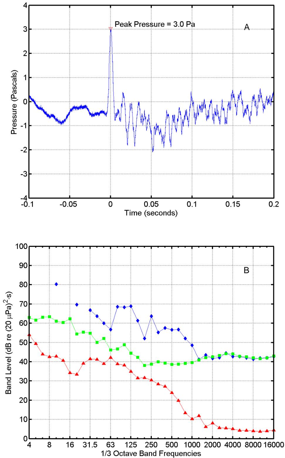
FIGURE C-38. (A) Pressure waveform and (B) one-third octave band levels for a RAM flight at 10:57 on 22 September 2004 recorded "Vizcaino Point". In (B),  $\diamond$  = missile sound energy;  $\square$  = instrumentation noise energy;  $\Delta$  = ambient noise power. Band frequencies in Hertz (Hz).
