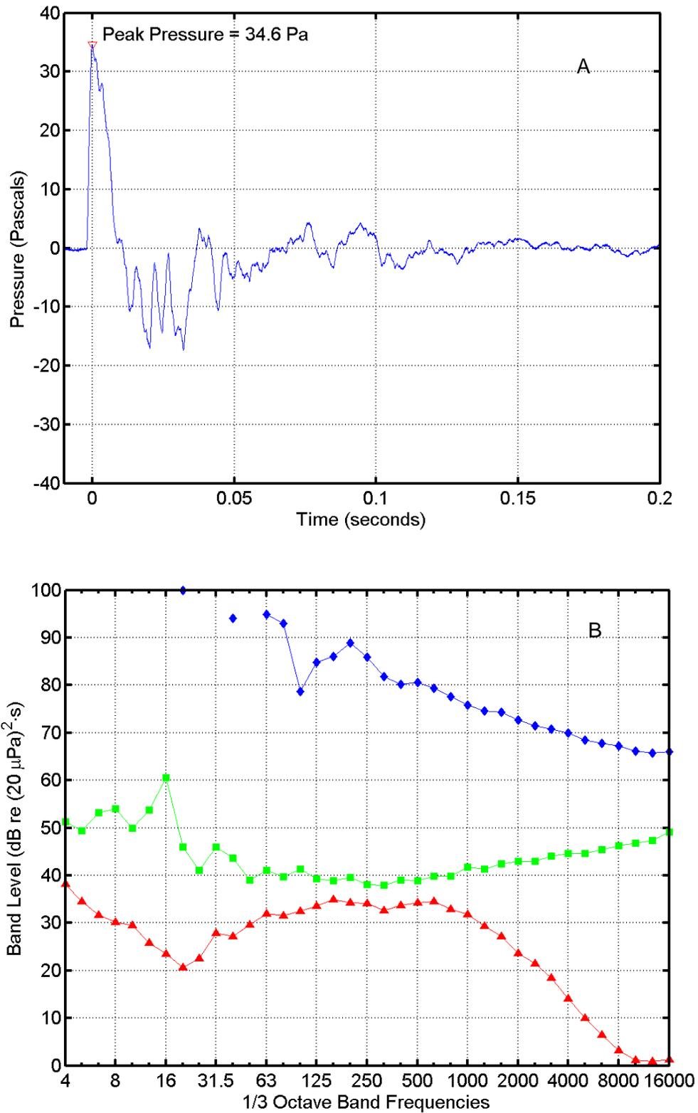
FIGURE C-22. (A) Pressure waveform and (B) one-third octave band levels for the AGS Slug launch at 15:43 on 26 July 2004 at "Bachelor Beach North". In (B),  $\diamond$  = missile sound energy;  $\square$  = instrumentation noise energy;  $\triangle$  = ambient noise power. Band frequencies in Hertz (Hz).
