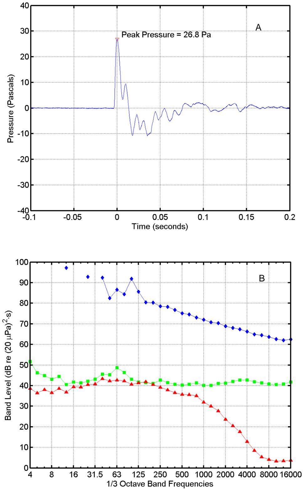
FIGURE C-47. (A) Pressure waveform and (B) one-third octave band levels for an AGS Missile flight at 13:29 on 27 January 2005 recorded at "Bachelor Beach North". In (B),  $\diamond$  = missile sound energy;  $\square$  = instrumentation noise energy;  $\Delta$  = ambient noise power.
