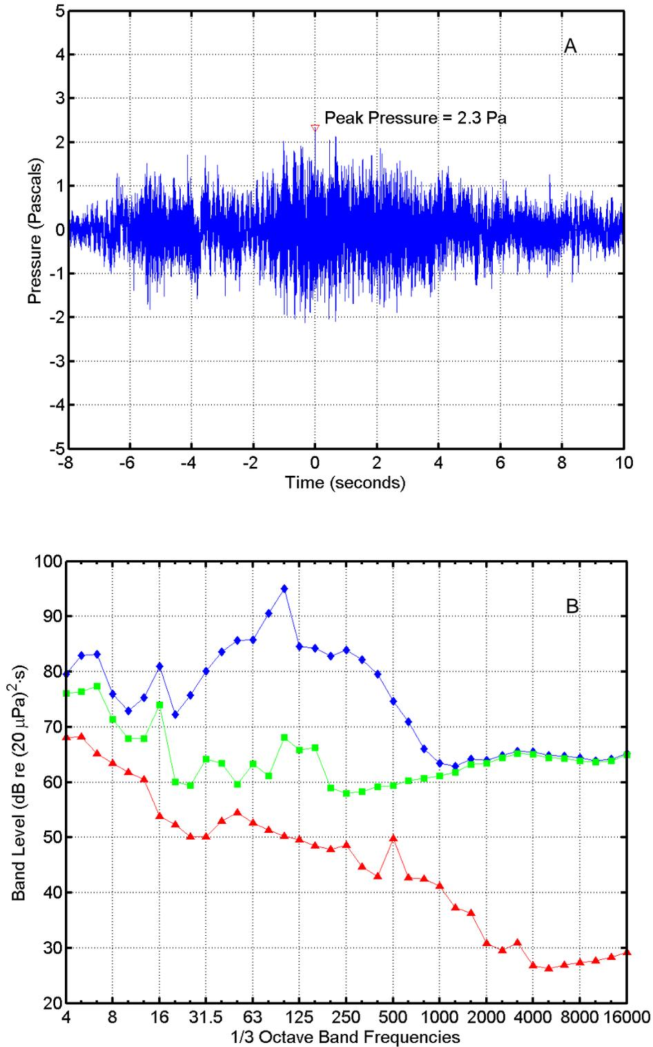
FIGURE C-25. (A) Pressure waveform and (B) one-third octave band levels for an Arrow flight at 10:20 on 29 July 2004 recorded "Vizcaino Point". In (B),  $\diamond$  = missile sound energy;  $\square$  = instrumentation noise energy;  $\Delta$  = ambient noise power. Band frequencies in Hertz (Hz).
