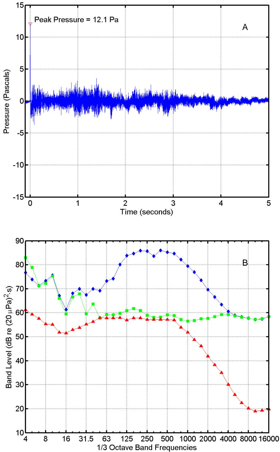
FIGURE C-4. (A) Pressure waveform and (B) one-third octave band levels for the second missile of the dual RAM launch at 11:46:12 on 5 May 2004 at "Bachelor Beach North". In (B),  $\diamond$  = missile sound energy;  $\square$  = instrumentation noise energy;  $\triangle$  = ambient noise power. Band frequencies in Hertz (Hz).
