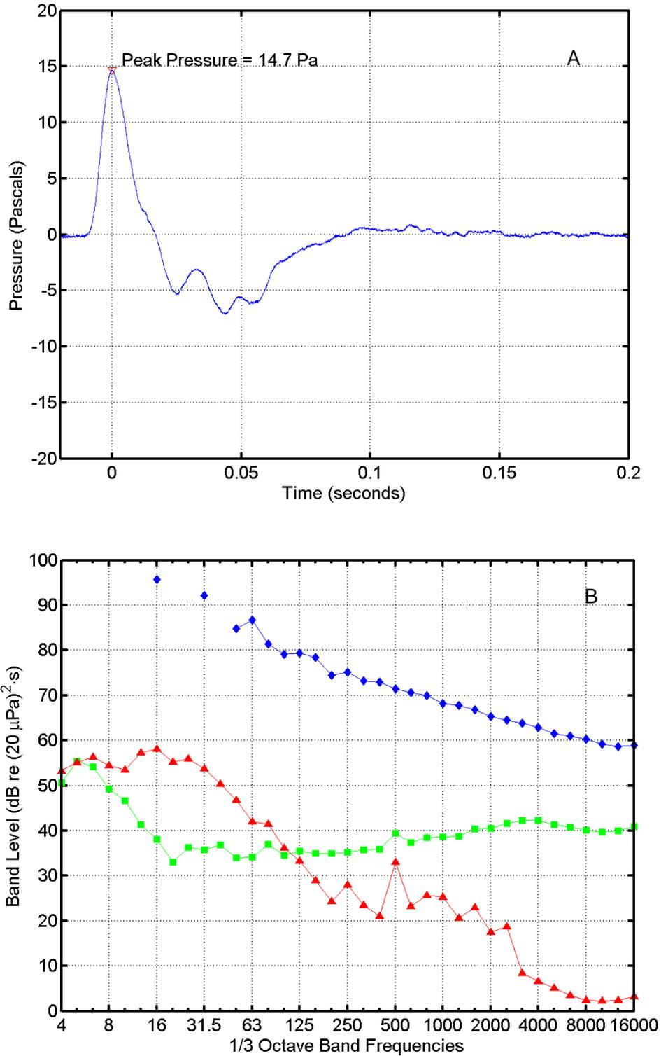
FIGURE C-20. (A) Pressure waveform and (B) one-third octave band levels for the AGS Slug launch at 15:10 on 26 July 2004 at "Vizcaino Point". In (B),  $\diamond$  = missile sound energy;  $\square$  = instrumentation noise energy;  $\Delta$  = ambient noise power. Band frequencies in Hertz (Hz).
