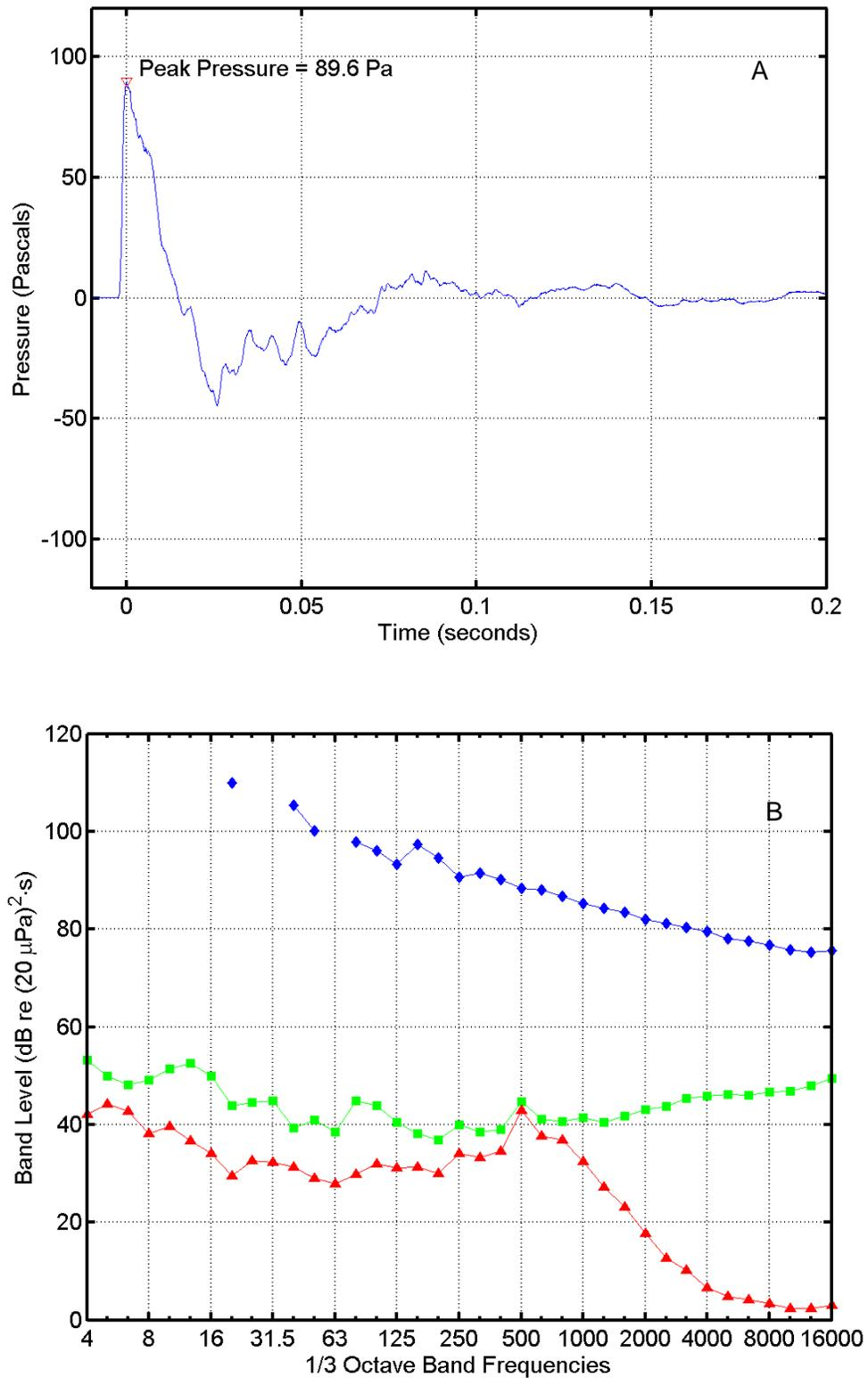
FIGURE C-21. (A) Pressure waveform and (B) one-third octave band levels for the AGS Slug launch at 15:10 on 26 July 2004 at "Dos Coves South". In (B),  $\diamond$  = missile sound energy;  $\square$  = instrumentation noise energy;  $\Delta$  = ambient noise power. Band frequencies in Hertz (Hz).
