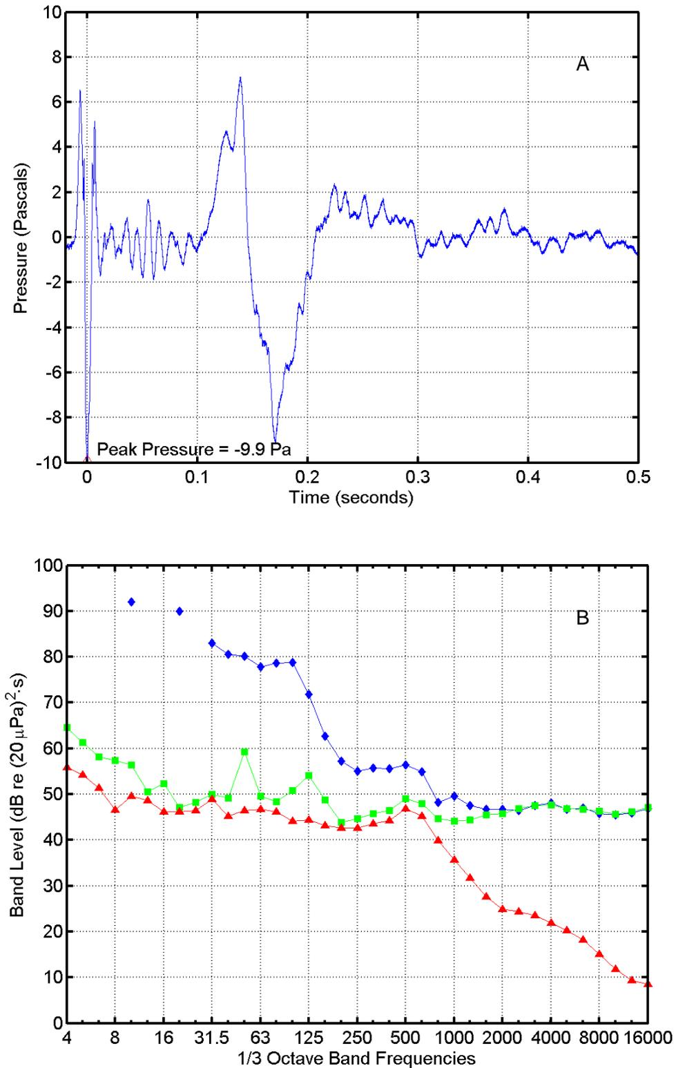
FIGURE C-18. (A) Pressure waveform and (B) one-third octave band levels for the AGS Missile launch at 15:08 on 3 June 2004 at "Dos Coves". In (B),  $\diamond$  = missile sound energy;  $\square$  = instrumentation noise energy;  $\Delta$  = ambient noise power. Band frequencies in Hertz (Hz).
