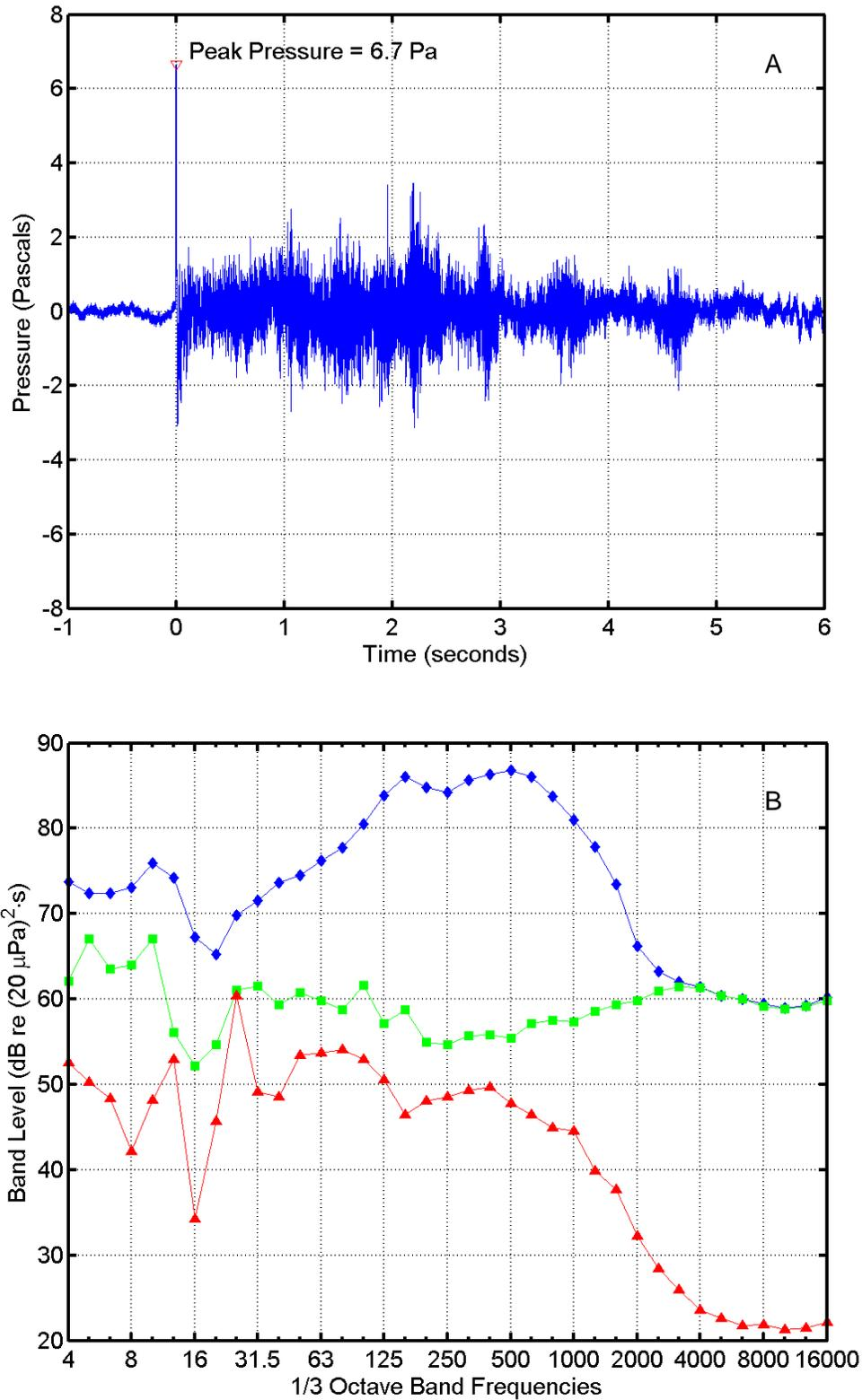
FIGURE C-37. (A) Pressure waveform and (B) one-third octave band levels for a RAM flight at 10:57 on 22 September 2004 recorded "Dos Coves South". In (B),  $\diamond$  = missile sound energy;  $\square$  = instrumentation noise energy;  $\Delta$  = ambient noise power. Band frequencies in Hertz (Hz).
