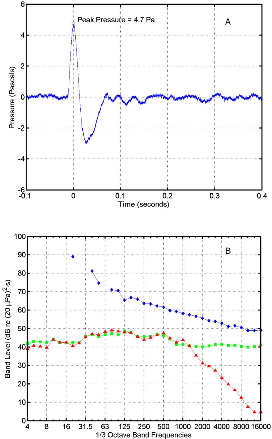
FIGURE C-46. (A) Pressure waveform and (B) one-third octave band levels for an AGS Slug flight at 11:41 on 27 January 2005 recorded at "Redeye I". In (B),  $\diamond$  = missile sound energy;  $\square$  = instrumentation noise energy;  $\Delta$  = ambient noise power. Band frequencies in Hertz (Hz).
