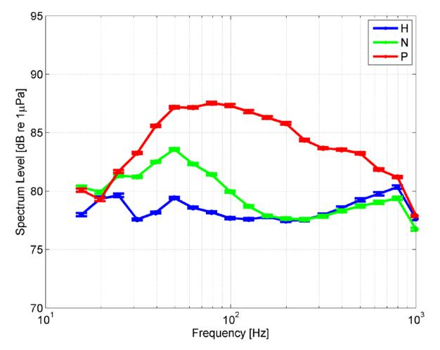
Figure 5. SOCAL Range Complex 1/3-octave bin average sound pressure spectrum levels over five years by site.
