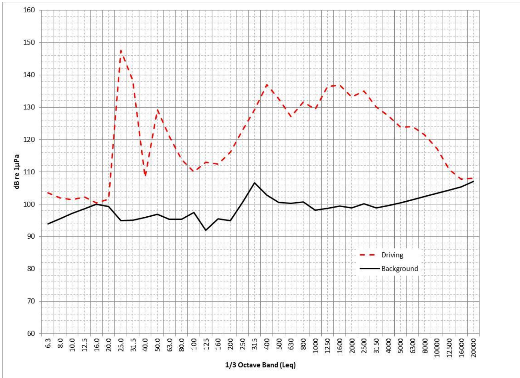
Figure B-7. 36-inch Steel Shell Piles with Vibratory Hammer 1 October, 2014
