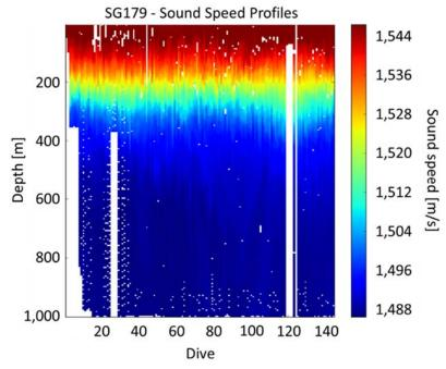
Figure 10: Sound-speed profiles recorded with SG179.
