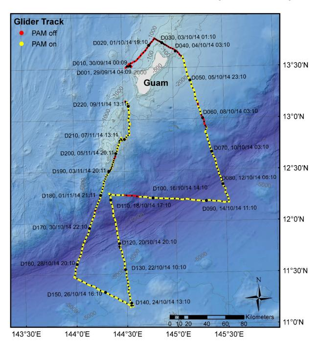
Figure 5: SG178 track line for the period 29 September–09 November 2014. Each black dot on the track line indicates the midpoint location of a glider dive; every 10<sup>th</sup> dive is represented by a larger dot. Labels indicate dive number (e.g., D001 for dive no. 1) and date/time (format: dd/mm/yy hh:mm UTC). Red sections indicate that the PAM system was OFF. The yellow marks indicate that the PAM system was active.
