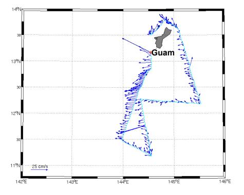
Figure 11: Depth-averaged currents measured with SG178.
