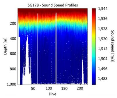
Figure 9: Sound-speed profiles recorded with SG178.
