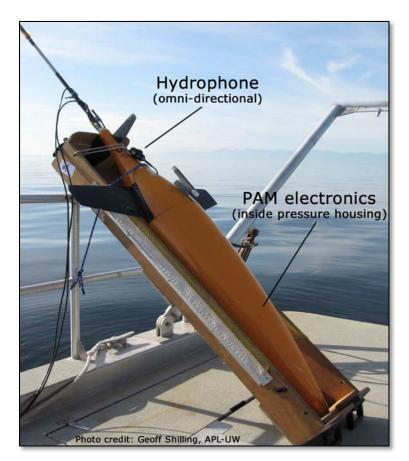
Figure 2: Passive-acoustic Seaglider. The Seaglider<sup>™</sup> is a commercial off-the-shelf instrument sold by Kongsberg, Inc. (Lynwood, WA, USA). The PAM system was developed and incorporated into the Seaglider by APL-UW (Seattle, WA, USA).
