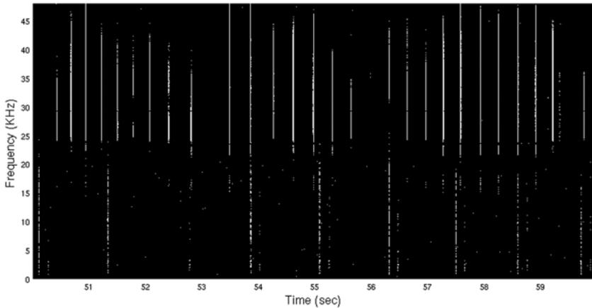
and processing speed limitations that prevent increasing either the time or frequency resolution of the full-band FFT processing. Also, M3R is intended to be a general system. The full-band resolutions of 46.875 Hz and 10.67 ms, while admittedly sub-optimal for some species, allow detection of a wide variety of odontocete vocalizations.
