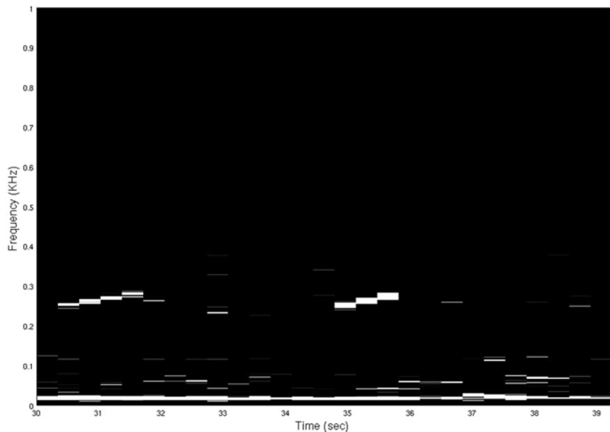
resolution in the band from 0 to 3 kHz. Again, each time-frequency bin of the spectrogram is compared to a time-varying threshold creating a binary detection spectrogram  $Q_{LF_i}(f,n)$  (Figure 4).
