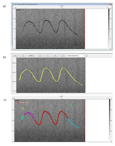
Figure 1. Example spectrograms of: (a) a dolphin whistle (without a contour outline); (b) contour manually traced and extracted using ROCCA; (c) traced and extracted automatically using the Whistle and Moan Detector (WMD) in PAMGuard, where different colors represent different individual whistles. In this example, WMD has labeled the sample whistle as four separate whistles, and false detections are shown in yellow, pink, and green.
