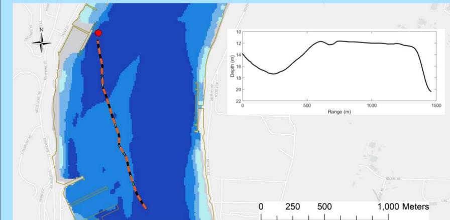
A small vessel (17 ft) slowly moved away from the pile (red dot). The dashed line shows the route followed while taking measurements of underwater noise from pile driving. Inset plot shows depth profile along the track. Measurements were taken over approximately 1 hr, during which ~1600 pile strikes were observed. Two piles approximately 5 m apart were used as the source (driven sequentially.)
