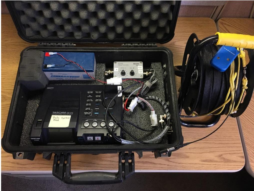
**Figure 3: Recording setup used for in situ near surface measurements from February 2016 to present. The five-pound weight for the hydrophone line is not pictured; the time depth recorder (in blue) is visible attached to the hydrophone line on the reel.**
