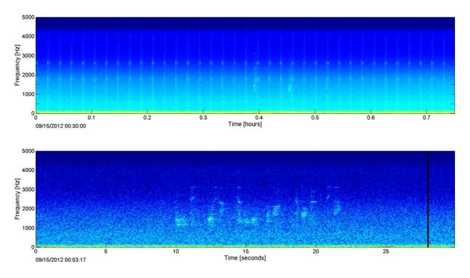
Figure 29. Underwater communications in the LTSA (top) and spectrogram (bottom) from a HARP recording site off the coast of Washington.
