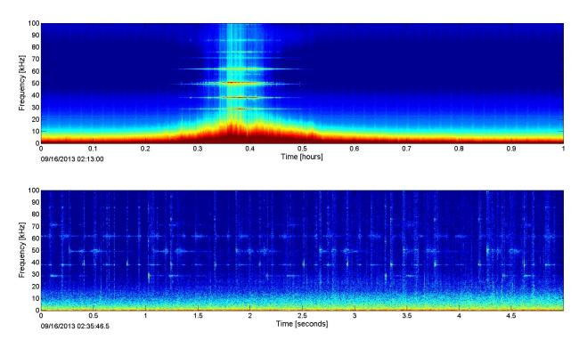
Figure 27. Example of an echosounder in the LTSA (top) and spectrogram (bottom) at site KO.
