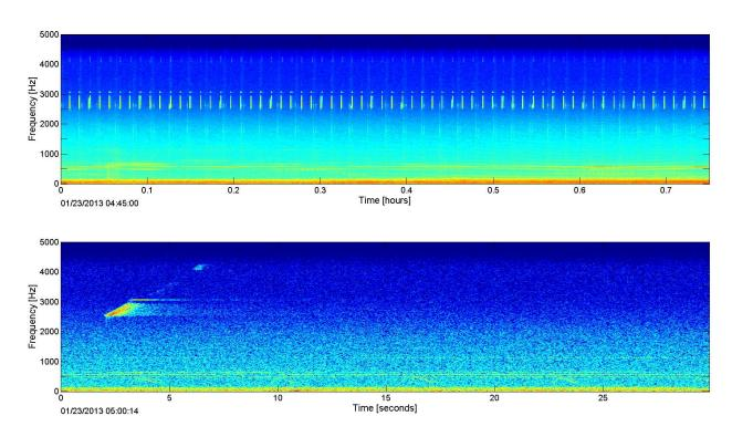
Figure 25. Example of MFA sonar in the LTSA (top) and spectrogram (bottom) from a recording site off the coast of Washington.
