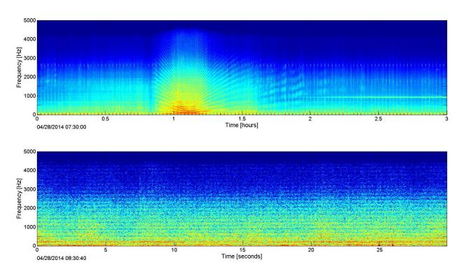
Figure 24. Broadband ship noise in the LTSA (top) and spectrogram (bottom) at site CB.
