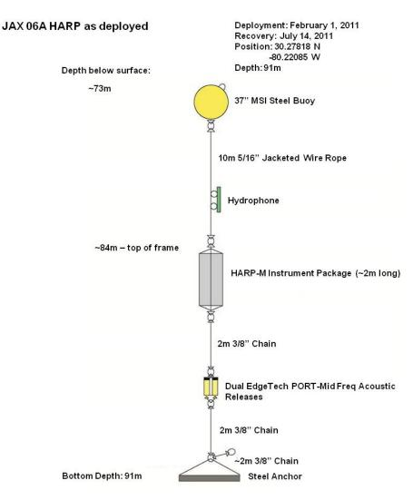
Figure 2. Schematic diagram showing details of the Jacksonville 06A HARP. Note that diagram is not drawn to scale.
