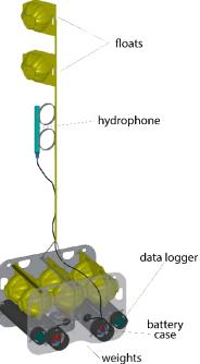
Figure 3. Schematic of a HARP seafloor package
