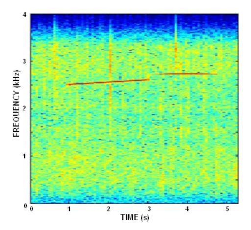
Figure 5. A spectrogram of a mid-frequency sonar ping at time between 1 and 3 seconds. The second shorter signal may be a reflection from the surface.
