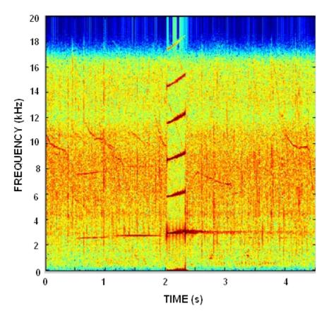
Figure 6. A sonar signal that saturated the EAR, producing many harmonics. Dolphin whistles can also be seen in the spectrogram. The peak-to-peak sound pressure level that causes EAR saturation is approximately 160 dB re 1 μPa.
